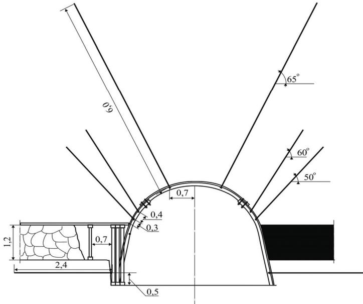
Fig. 3. Recommended scheme of maintaining the prefabricated drift
