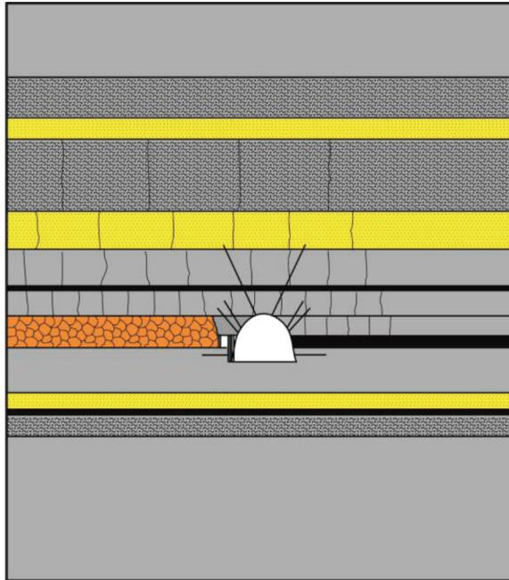
Fig. 2. General geomechanical model for the research into the stability of prefabricated drift
