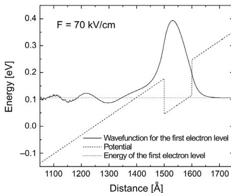
Fig. 6. Wavefunction for the first electron level (solid line), shape of QW potential (dashed line) and the energy of the first electron level (dotted line) obtained on the basis of theoretical calculations performed for a InGaAs/GaAs QW under the electric field of 70 kV/cm.
