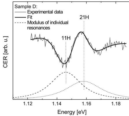
Fig. 4. Fit and resonance associated with 11H and 21H transitions for sample *D*.
