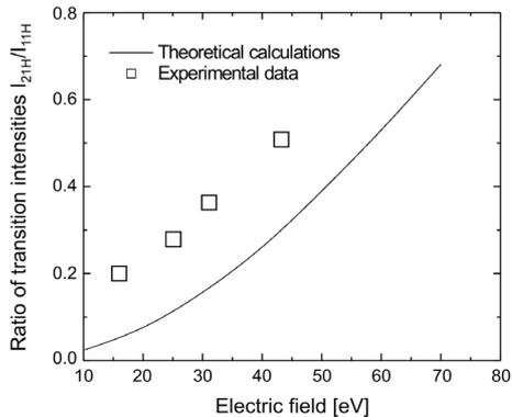
Fig. 5. Ratio of intensity of 21H transition to intensity of 11H transition as a function of electric field.
