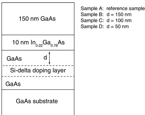
Fig. 1. Layer structure of the samples.
