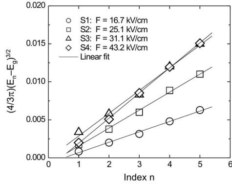
Fig. 3. Built-in electric field determined from FKO period.
