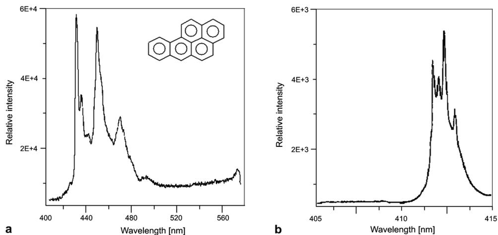
Fig. 7. Room temperature low resolution fluorescence spectrum (a) and low temperature ( $-150^\circ\text{C}$ ) high resolution fluorescence spectrum (b) of  $2.0 \times 10^{-5}$  g/l benzo(a)pyrene in n-heptane ( $\lambda_{\text{exc}} = 337$  nm).
