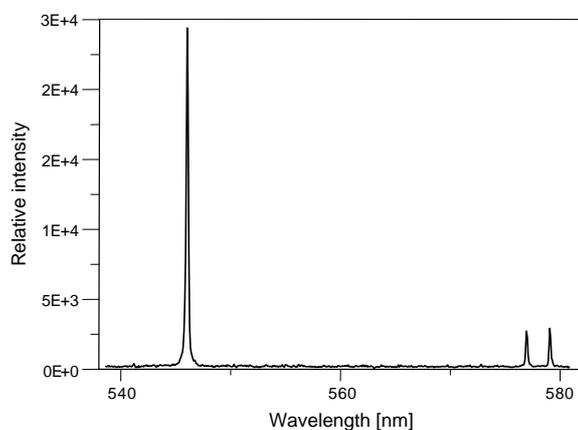
Fig. 5. Mercury spectral lines acquired using the high resolution grating (300 grooves/mm).
