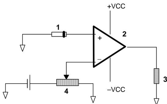
Fig. 4. Temperature controller circuit diagram: 1 – semiconductor diode, 2 – operational amplifier, 3 – power resistor, 4 – potentiometer.
