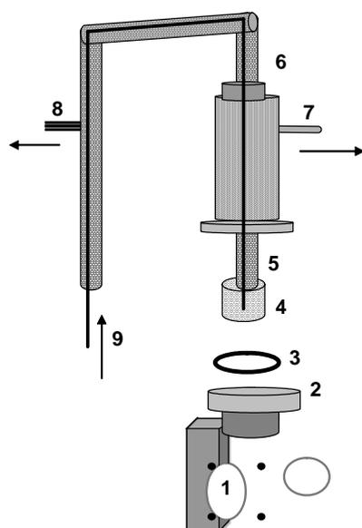
Fig. 2. Open cycle liquid nitrogen cryostat: 1 – aluminum block with quartz windows, 2 – Varian type adapter, 3 – Rubber O-ring, 4 – metal block with drilled volume to receive liquid nitrogen and to act as a heat exchanger, 5 – liquid nitrogen transfer line, 6, 7 – stainless steel cylinder with vacuum outlet, 8 – vacuum outlet to evacuate the transfer line, 9 – capillary tube for liquid nitrogen inlet.
