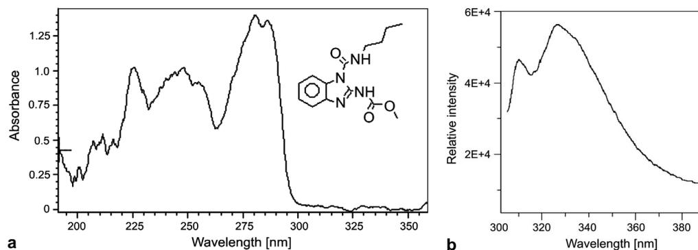
Fig. 8. Absorption spectrum (a) and fluorescence spectrum (b) of  $1 \times 10^{-3}$  M benomyl in  $\text{CH}_3\text{CN}$ , ( $\lambda_{\text{exc}} = 290$  nm).
