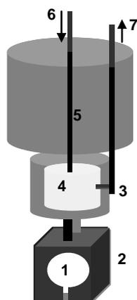
Fig. 3. Liquid nitrogen transfer line and sample cell block: 1 – sample volume drilled into the metal block with quartz window in the front, 2 – metal block from stainless steel, 3 – metal block with drilled volume 4 to receive liquid nitrogen to act as a heat exchanger, 4 – metal tube through which liquid nitrogen is removed, 5 – copper cylinder evacuated all over the transfer line, 6, 7 – liquid N<sub>2</sub> inlet and outlet.
