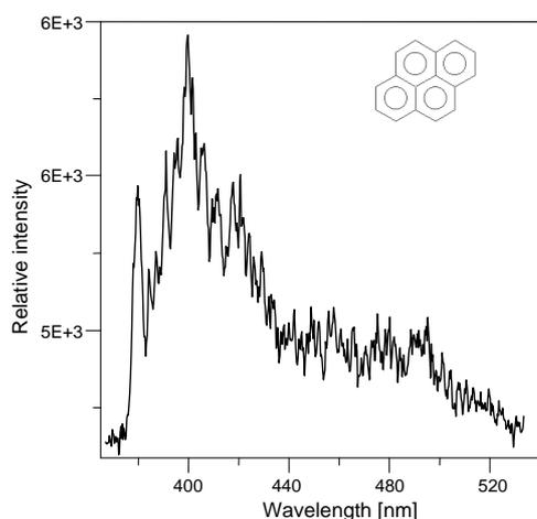
Fig. 6. Fluorescence spectrum of  $1.0 \times 10^{-6}$  g/l pyrene in cyclohexane at room temperature obtained with a single 15 nsec duration laser pulse at 337.1 nm using  $N_2$  laser excitation source.
