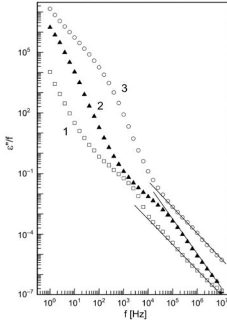
▲ Fig. 2. Frequency dependences of  $\varepsilon''/f$  at 370 K (curve 1), 423 K (curve 2) and 488 K (curve 3).
