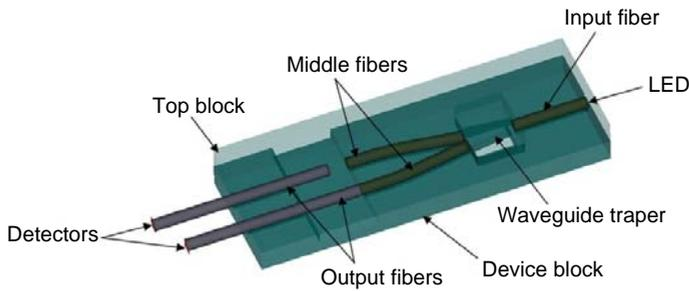
Fig. 5. 3D model of the acrylic-based asymmetric Y-branch POF coupler for device simulation.
