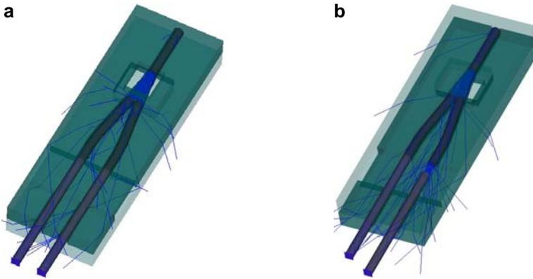
Fig. 7. 3D ray tracing layout of acrylic-based asymmetric Y-branch POF coupler: fibers non-displaced (a), and shifted output fiber (b).
