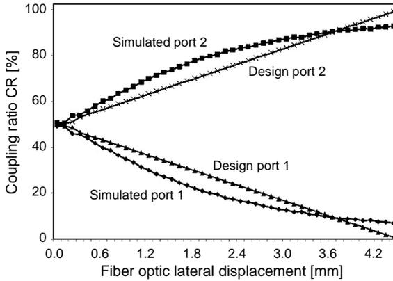
Fig. 8. Coupling ratio against output fiber lateral displacement for asymmetric Y-branch POF coupler.
