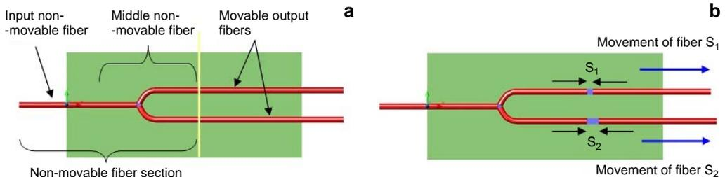
Fig. 2. Generic Y-branch coupler with movable output fibers, showing lateral displacement of  $S_1$  (a) and  $S_2$  (b).
