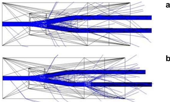
Fig. 6. 2D ray tracing layout of acrylic-based asymmetric Y-branch POF coupler: fibers non-displaced (a), and shifted output fiber (b).
