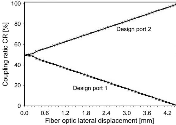
Fig. 3. Coupling ratio against output fiber lateral displacement for asymmetric Y-branch POF coupler.
