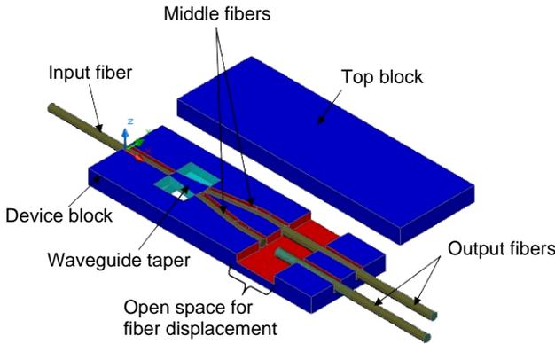
Fig. 4. CAD design for acrylic-based asymmetric Y-branch POF coupler.
