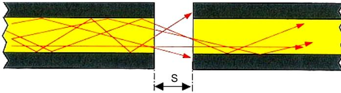
Fig. 1. Attenuation induced by lateral displacement of two fibers [1].
