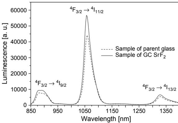
Fig. 7. Luminescence spectra of glass AW3 doped with Nd<sup>3+</sup> ions.
