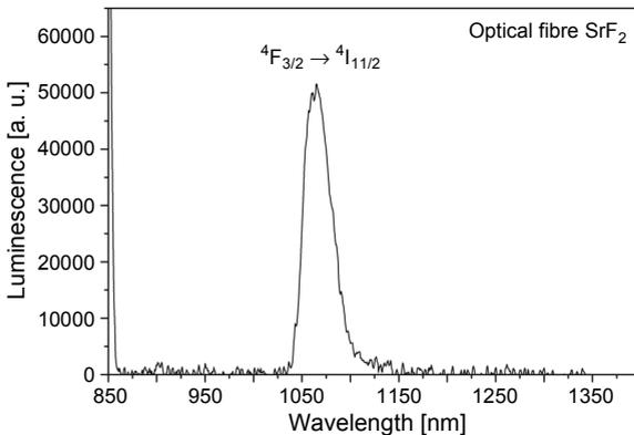
Fig. 8. Luminescence spectra of optical fibre (SiO<sub>2</sub>–Al<sub>2</sub>O<sub>3</sub>–ZnO–Na<sub>2</sub>O–SrF<sub>2</sub>) doped with Nd<sup>3+</sup> ions.
