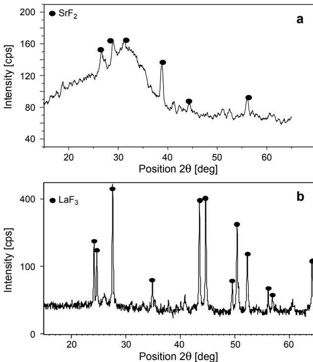
Fig. 2. XRD patterns of glasses after the heat treatment: glass AW3 635 °C/30 min (a), glass AW1 563 °C/30 min (b).
