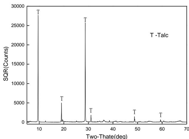
Fig. 1. The XRD spectra of talc
