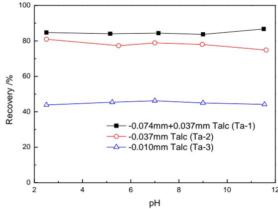
Fig. 3. Effects of pH values on flotation behavior of talc with different particle size (PAX=1×10<sup>-4</sup> mol/ dm<sup>3</sup>, MIBC=9 mg/ dm<sup>3</sup>)
