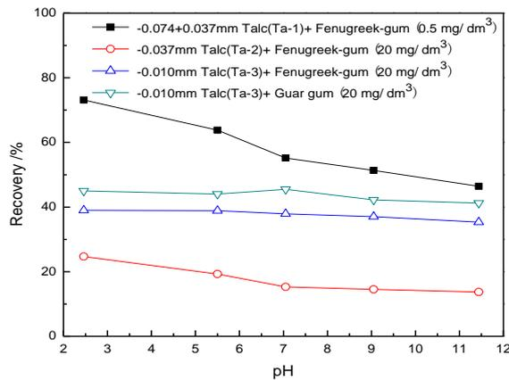
Fig. 4. Effects of FG on flotation behavior of talc with different particle size as a function of pH (PAX=1×10<sup>-4</sup> mol/ dm<sup>3</sup>, MIBC=9 mg/ dm<sup>3</sup>)
