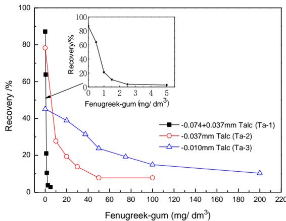
Fig. 5. The effect of FG concentration on flotation behavior of talc with different particle size (pH=5.5, PAX=1×10<sup>-4</sup> mol/ dm<sup>3</sup>, MIBC=9 mg/ dm<sup>3</sup>)
