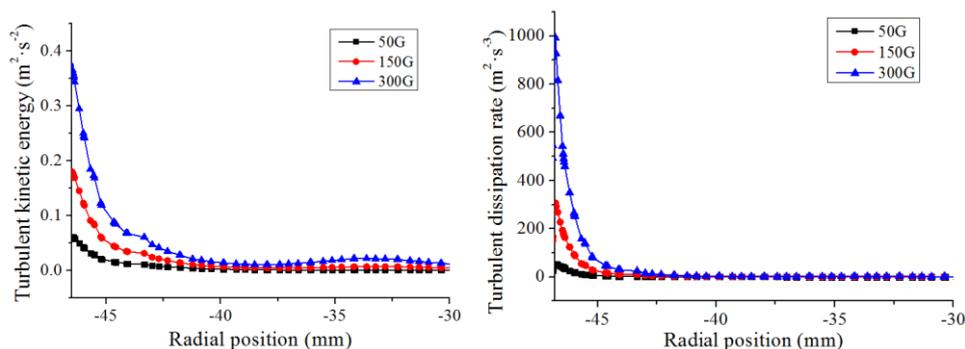
Fig. 6. Effect of centrifugal force on radial turbulence
