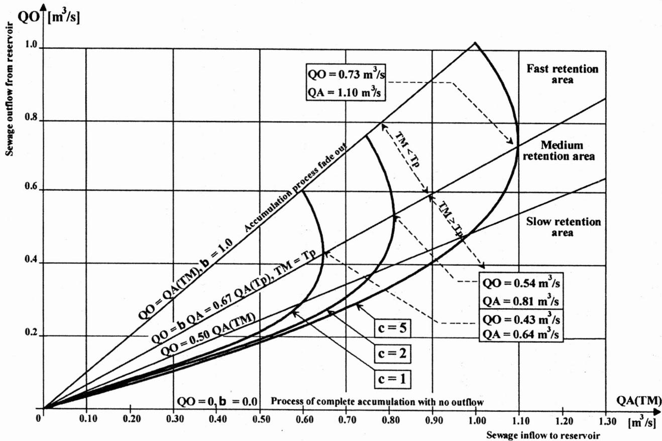
Fig. 3. Determination of traditional reservoirs' storage areas dependent on flow reduction rate
