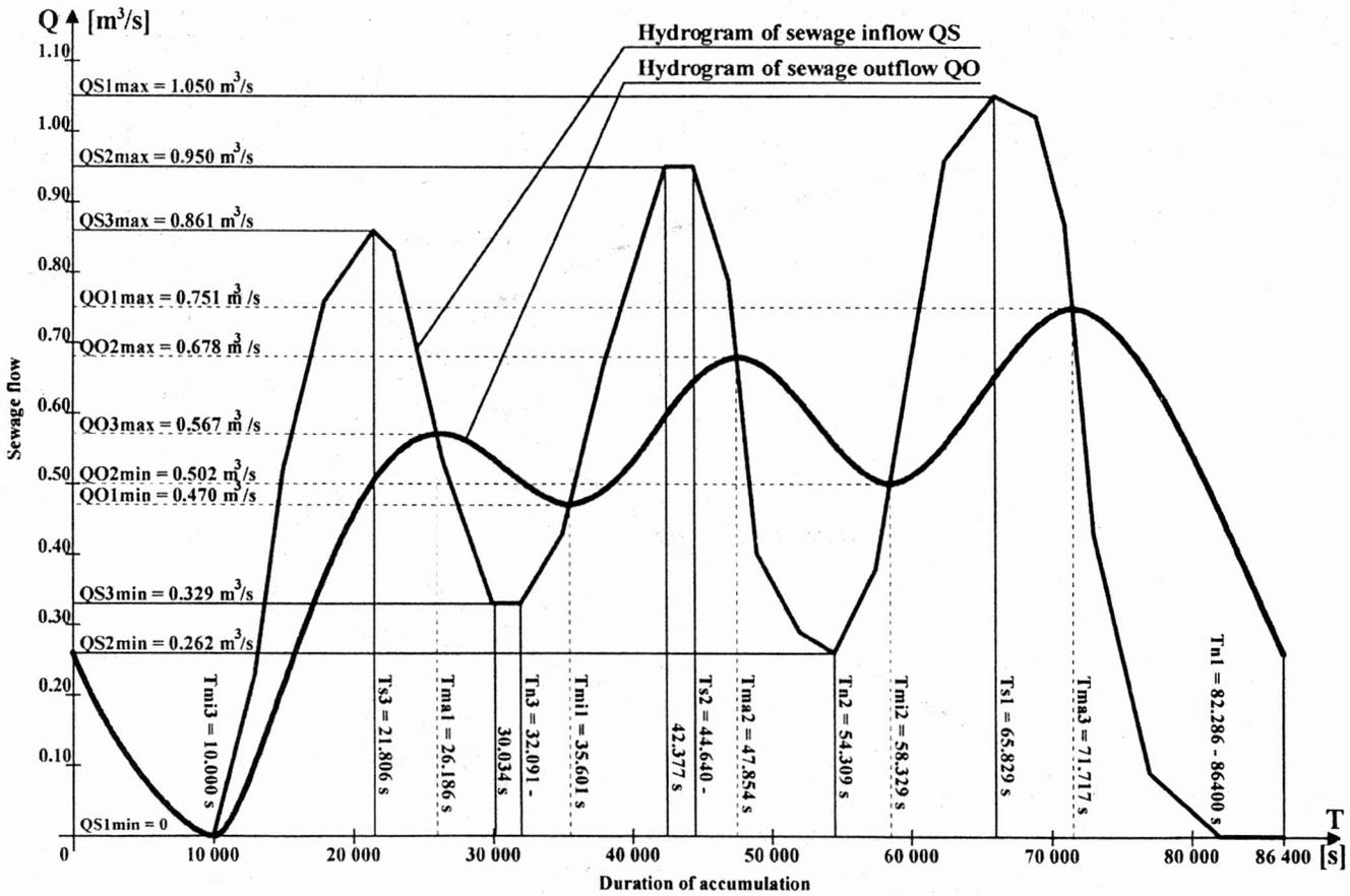
Fig. 1. Outflow hydrogram of a traditional reservoir determined by means of numerical program for a given inflow hydrogram
