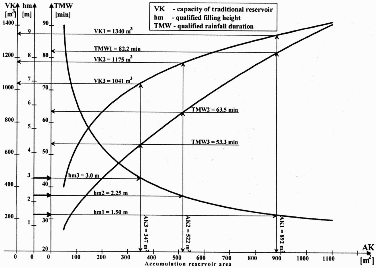
Fig. 2. Qualified rainfall duration and required reservoir capacity versus maximum filling height at various horizontal levels of traditional reservoirs
