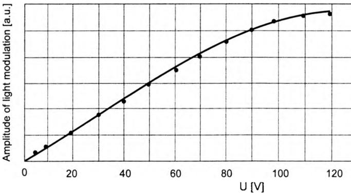
Fig. 3. Amplitude of light modulation vs. applied voltage for PDLC containing  $SmC_A^*$  phase of W-104 at  $30\text{ }^\circ\text{C}$ , mean droplet volume  $\sim 15\text{ }\mu\text{m}^3$ , mean droplet aspect ratio  $\sim 8$ .
