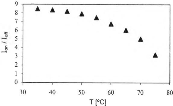
Fig. 5. Optical contrast *vs.* temperature for PDLC film containing 20% by weight of W-101A mixture; film thickness 8  $\mu\text{m}$ , mean droplet volume  $\sim 15 \mu\text{m}^3$ , mean droplet aspect ratio 10.
