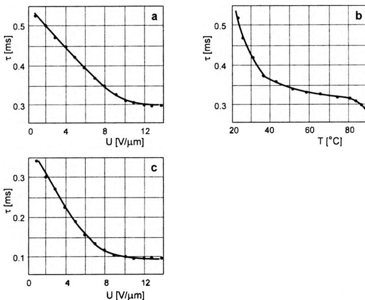
Fig. 8. Dependence of total switching time PDLC containing:  $\text{SmC}_\Lambda^*$  phase of W-104 mixture on: a – applied voltage (at  $T = 30$  °C), b – temperature (at  $U = 4$  V), c –  $\text{SmC}^*$  of the same mixture on applied voltage,  $T = 85.5$  °C; film thickness  $8 \mu\text{m}$ , mean droplet volume  $\sim 15 \mu\text{m}^3$ , mean aspect ratio  $\sim 10$ .
