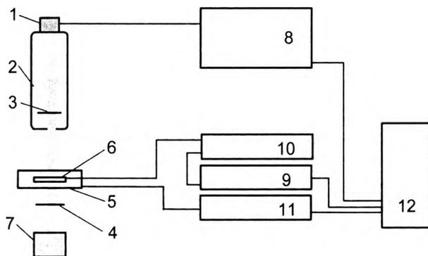
Fig. 1. Block scheme of the electro-optic measuring set-up: 1 – silicone diode photodetector, 2 – polarizing microscope, 3 – analyzer, 4 – polarizer, 5 – hot stage, 6 – PDLC sample, 7 – halogen lamp, 8 – oscilloscope, 9 – signal generator, 10 – voltage amplifier, 11 – hot-stage driver, 12 – driving PC.
