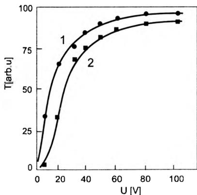
Fig. 9. Static electro-optical characteristics of PDLC containing: 1 – W-104 and 2 – W-101 mixtures;  $T = 40$  °C; film thickness  $8 \mu\text{m}$ , mean droplet volume  $\sim 15 \mu\text{m}^3$ , mean aspect ratio  $\sim 10$ .
