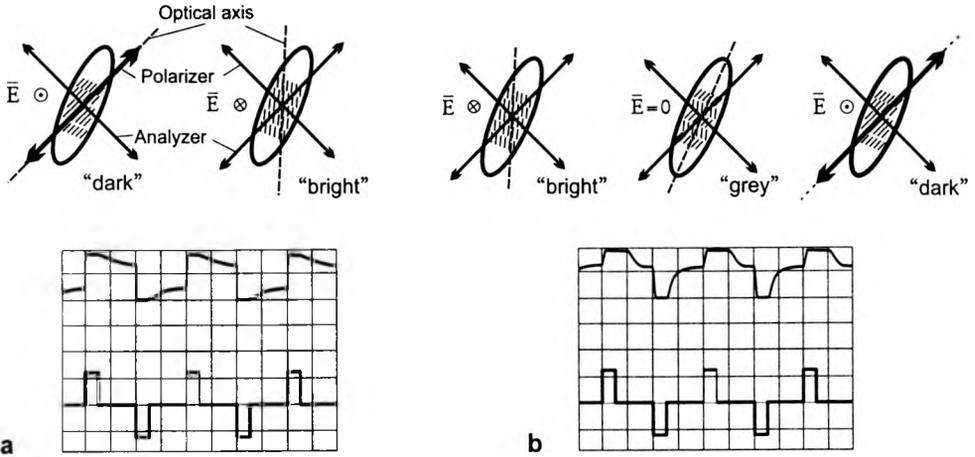
Fig. 2. Schematic oscilloscope view of saturated electro-optical switching of PDLC containing W-104 mixture by 100 Hz signal. Bistable switching of  $SmC^*$  phase at  $85.5\text{ }^\circ\text{C}$  (a), tristable switching of  $SmC_A^*$  phase at  $75\text{ }^\circ\text{C}$  (b), mean droplet volume  $\sim 15\text{ }\mu\text{m}^3$ , mean droplet aspect ratio  $\sim 10$ .
