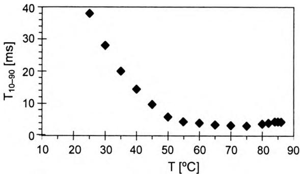
Fig. 7. Response time of PDLC film containing 20% b.w. of W-101A mixture vs. temperature; film thickness 8  $\mu\text{m}$ , mean droplet volume  $\sim 15 \mu\text{m}^3$ , mean droplet aspect ratio 10.
