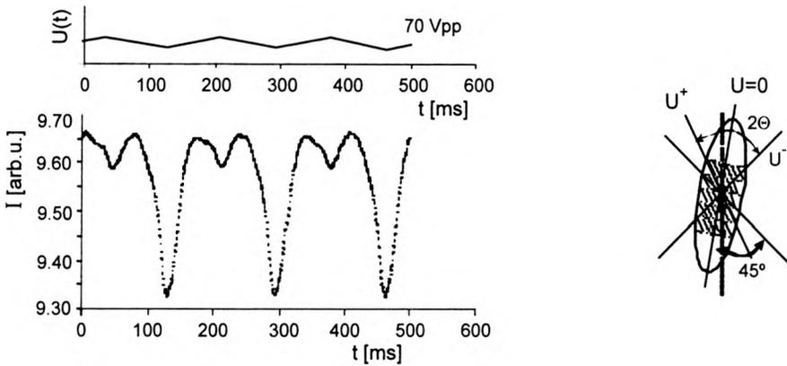
Fig. 6. Electro-optical response to triangle signal of PDLC film containing 20% bw. of W-101 mixture measured at room temperature; film thickness  $8 \mu\text{m}$ , mean droplet volume  $\sim 15 \mu\text{m}^3$ , mean droplet aspect ratio 10.
