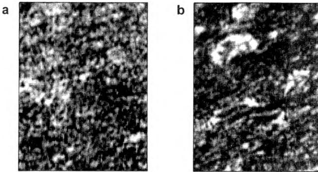
Fig. 4. Microscopic view of the PDLC film containing  $\text{SmC}_A^*$  phase of W-104 at 75 °C. **a** – off-state, **b** – on state; film thickness 8  $\mu\text{m}$ , mean droplet volume  $\sim 15 \mu\text{m}^3$  mean droplet aspect ratio 8.
