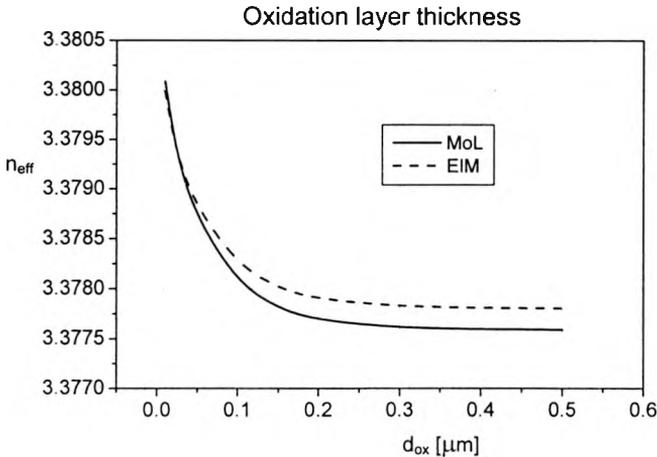
Fig. 4. Impact of the aperture width  $d_{\text{ox}}$  on the effective index  $n_{\text{eff}}$  calculated with the aid of the MoL and EIM.
