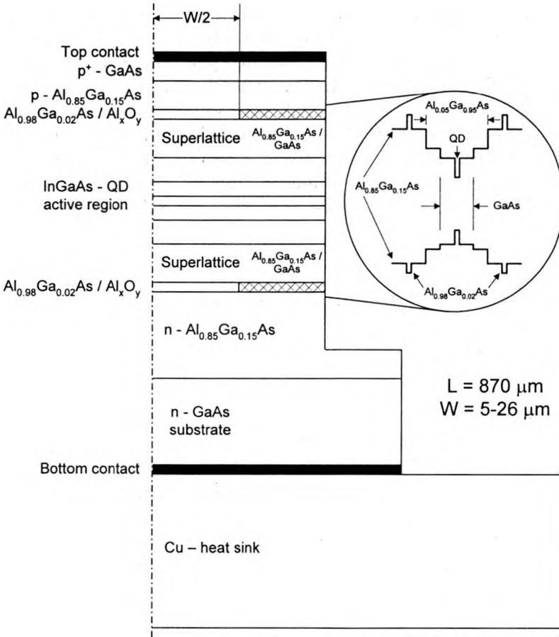
Fig. 1. Structure of 1.3- $\mu\text{m}$  quantum-dot (QD) (InGa)As/GaAs edge-emitting diode laser.  $L$  and  $W$  – length and width, respectively, of the active region.
