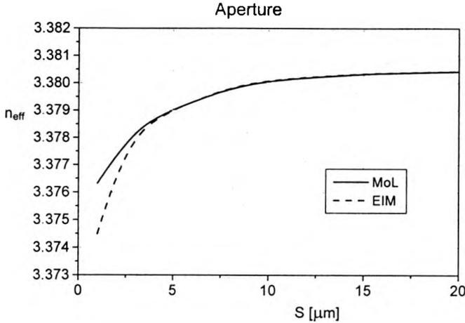
Fig. 3. Impact of the aperture width  $W$  on the effective index  $n_{\text{eff}}$  with calculated the aid of the MoL and EIM.
