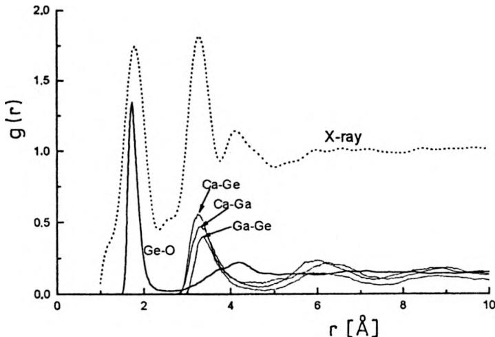
Fig. 6. Pair distribution functions for glasses of  $\text{Ca}_3\text{Ga}_2\text{Ge}_3\text{O}_{12}$  composition: dotted line — X-ray scattering method, solid lines — MD simulation, several partial PDFs.
