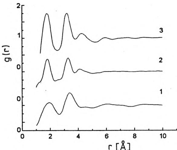
Fig. 4. Pair distribution functions for glasses of  $\text{Ca}_3\text{Ga}_2\text{O}_6$  (1),  $\text{Ca}_3\text{Ga}_2\text{Ge}_3\text{O}_{12}$  (2), and  $\text{Ca}_3\text{Ga}_2\text{Ge}_4\text{O}_{14}$  compositions.
