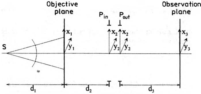
Fig. 4. Pupil representation of the simplified optical system.
