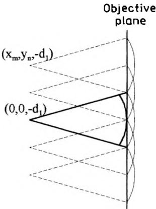
Fig. 2. Transformation of a spherical wave emerging from a point source on the axis and incident on the even amplitude object structure (objective plane).
