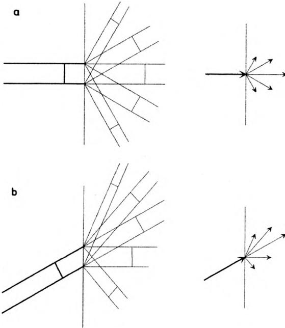
Fig. 3. Transformation of a plane wave incident on the even amplitude object structure: a — for a plane wave propagating along the optical axis, b — for the plane incident at an angle with respect to the optical axis.
