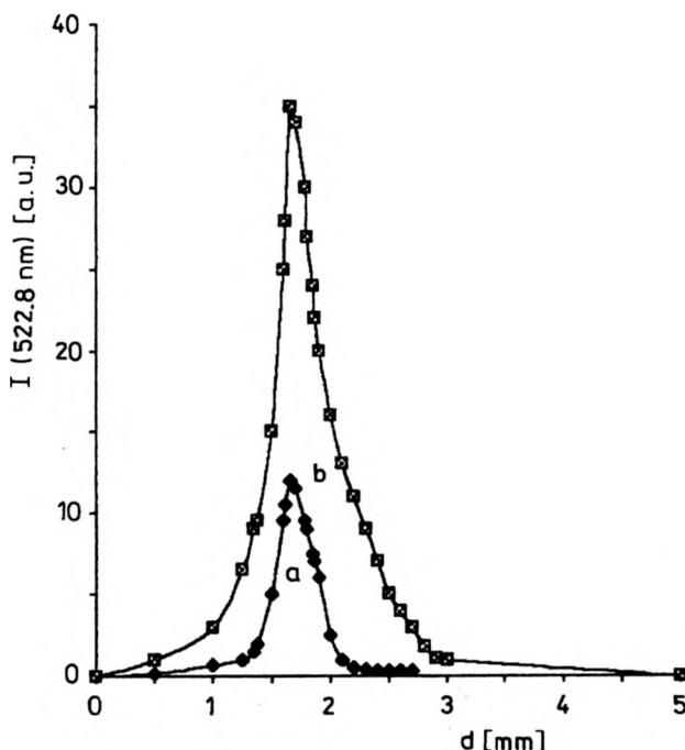
Fig. 2. Absorption of 522.75 nm radiation vs. the distance from the end of the small capillary: a – without magnetic field, b – with the magnetic field.
