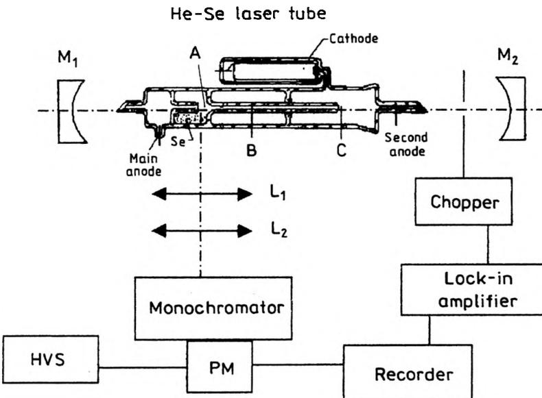
Fig. 1. Experimental set-up for lock-in signal analysis.  $M_1$ ,  $M_2$  – laser mirrors,  $L_1$ ,  $L_2$  – optical lenses, HVS – high voltage supply, PM – photomultiplier.
