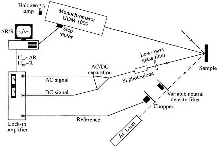
Fig. 1. Scheme of the set-up for photoreflectance measurements.
