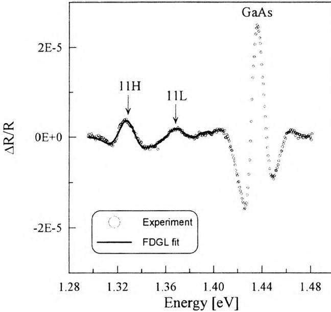
Fig. 2. Room temperature PR spectrum of  $\text{In}_{0.115}\text{Ga}_{0.885}\text{As}/\text{GaAs}$  MQW. Open circles — experiment, solid line — fit according to the first derivative of Gaussian lineshape.
