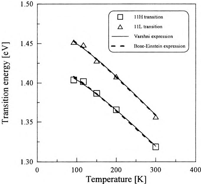
Fig. 4. Temperature dependence of energy of 11H (rectangles) and 11L (triangles) transitions. Solid line – fit according to the Varshni expression (Eq. (2)), dashed line – fit according to the Bose–Einstein expression (Eq. (3)).
