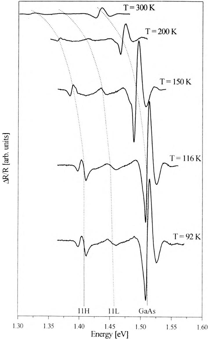
Fig. 3. PR spectra of  $\text{In}_{0.115}\text{Ga}_{0.885}\text{As}/\text{GaAs}$  MQW as a function of temperature in the range 92–300 K.
