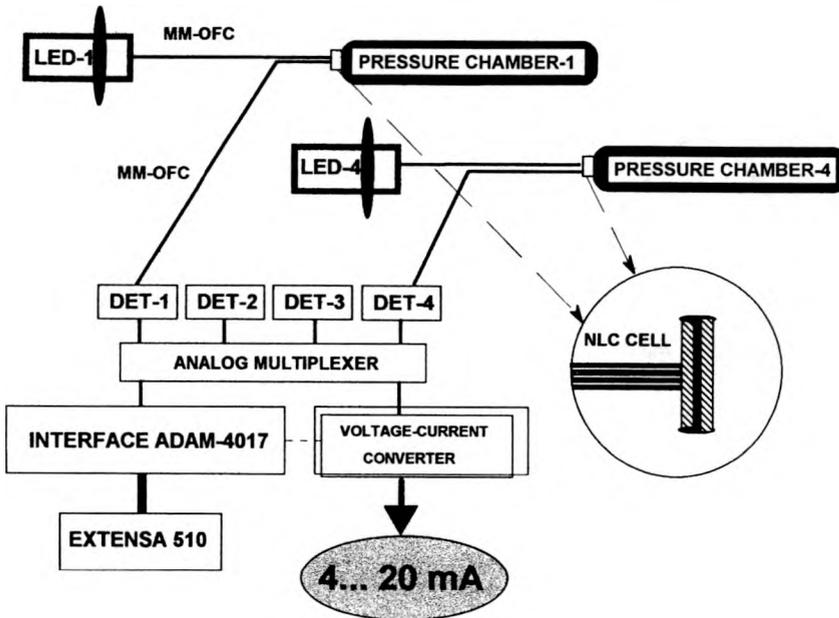
Fig. 2. Multiplexed fiber-optic sensor for continuous pressure monitoring based on nematic cells with an interface ADAM-4017 connected with a portable computer Extensa-510 and voltage current converter (MM-OFC – multimode fiber cable, LED-1(4) – light emitting diodes).
