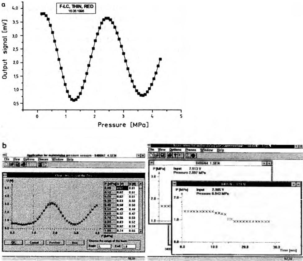
Fig. 4. Pressure characteristics of the sensor in the Frederiks configuration (a) and measurement of time-dependent pressure variations by using the field LC sensor (b).
