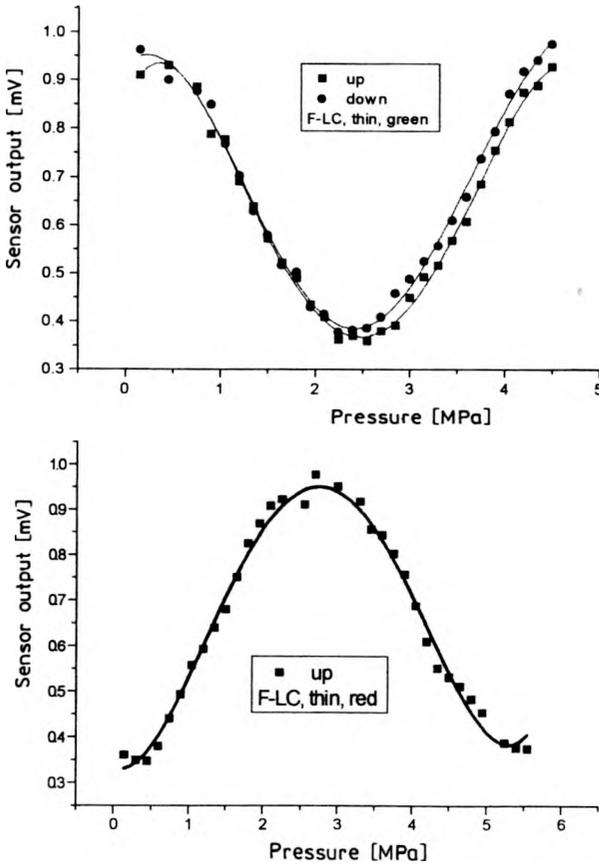
Fig. 3. Calibration of the liquid crystal pressure sensor in Frederiks configuration (F-LC) for red (crossed polarizers) and green (parallel polarizers) cells.
