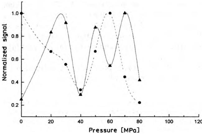
Fig. 9. Pressure characteristics of a radially and planar oriented liquid crystal fiber with a single-mode lead-in fiber and a multimode lead-out fiber up to 80 MPa. 30- $\mu$ m capillary filled up with two different nematics ( $\lambda = 633$  nm).  $\blacktriangle$  – radial structure,  $\varphi = 30$   $\mu$ m, LC1110,  $\bullet$  – planar structure,  $\varphi = 30$   $\mu$ m, LC1115.
