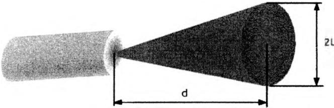
Fig. 6. Geometrical illustration for numerical aperture ( $d$  – distance from fiber to the light spot,  $L$  – radius of the light spot).
