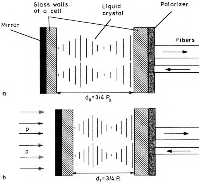
Fig. 1. Operation principle of the pressure sensor in the reflective configuration under atmospheric pressure (a) and under hydrostatic pressure (b).
