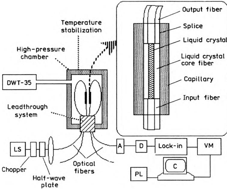
Fig. 7. Experimental setup of the fiber-optic liquid crystal pressure sensor in all-optical configuration. D – detector, VM-DC – voltmeter, C – computer, PL – plotter.
