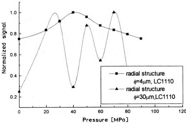
Fig. 8. Pressure characteristics of the radially oriented liquid crystal fiber with single mode lead-in fiber and a multimode lead-out fiber up to 100 MPa; 30- $\mu$ m and 4- $\mu$ m capillary filled up with nematics ( $\lambda = 633$  nm).
