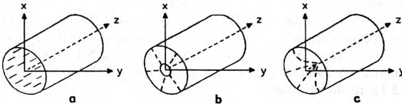
Fig. 5. Types of alignment of the LC director inside the fiber: a – planar structure, b – radial structure, c – axial structure.
