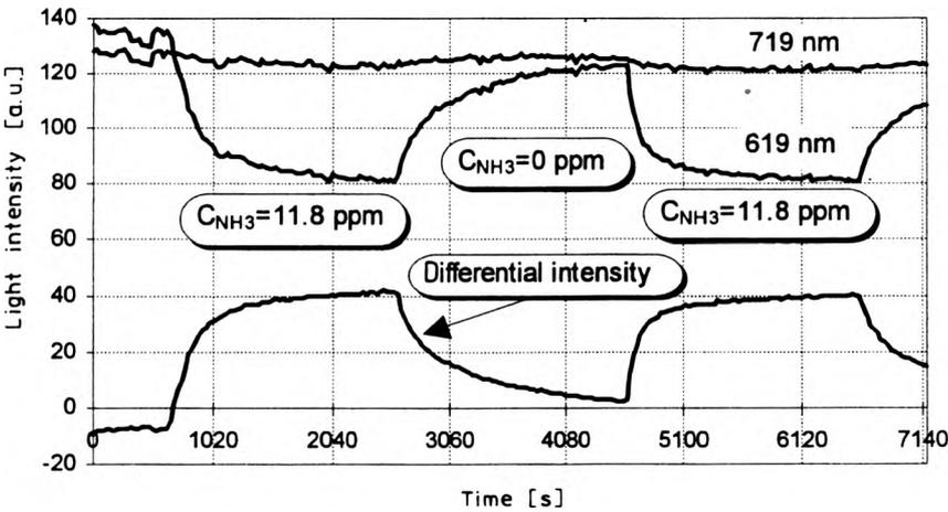
Fig. 5. Changes in light intensity for the selected wavelengths caused by the presence of ammonia vapours.
