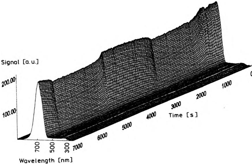
Fig. 4. Evolution involving the light spectrum leaving the sensor effected by the periodic action of air and ammonia vapours of the concentration 11.8 ppm.
