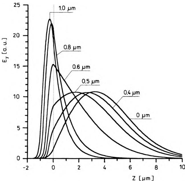
Fig. 2. Influence of the sensor layer thickness on the distribution of the electrical field of the zero order mode.
