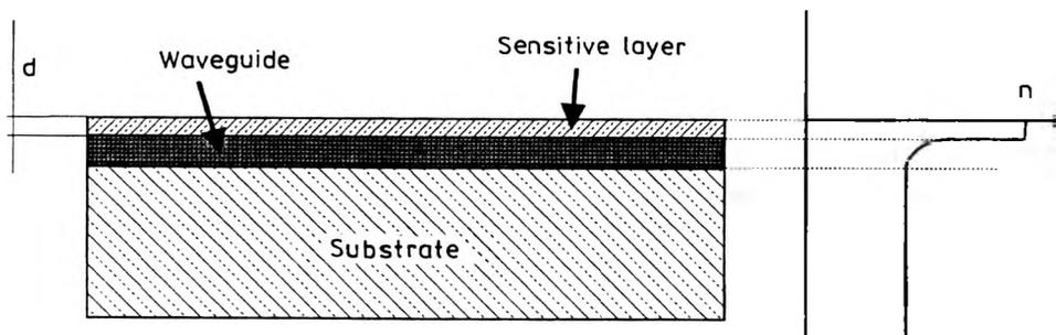
Fig. 1. Diagram of the investigated structure of the waveguide sensor layer.
