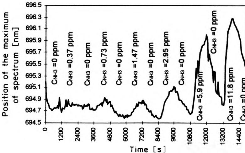
Fig. 6. Influence of ammonia concentration on the position of spectrum maximum of the sensor layer.
