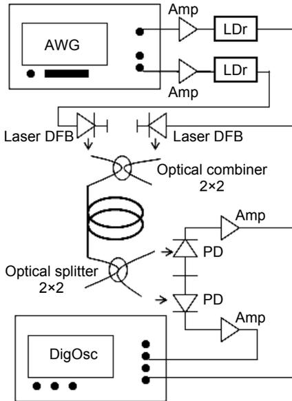
◀ Fig. 3. Block scheme of the experimental setup.
