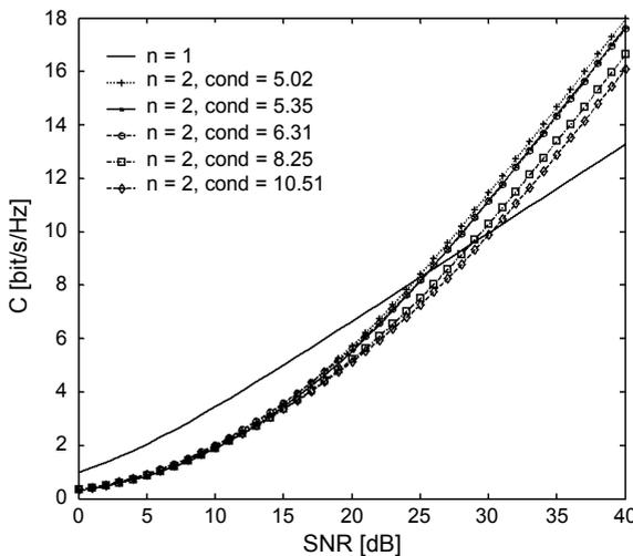
Fig. 4. Real maximum spectral efficiencies calculated according to Eq. (7) against SNR of a single channel system for different real  $2 \times 2$  MIMO system matrices that have various condition numbers (cond).
