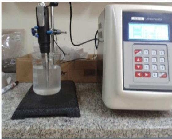
Fig. 2. XO-800S Ultrasonic homogenizer
