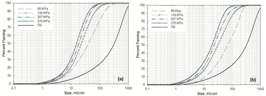
Fig. 2. Cumulative passing plots of products for -710 micrometer feed comminuted at different operational pressures; feed material is abbreviated FM.
