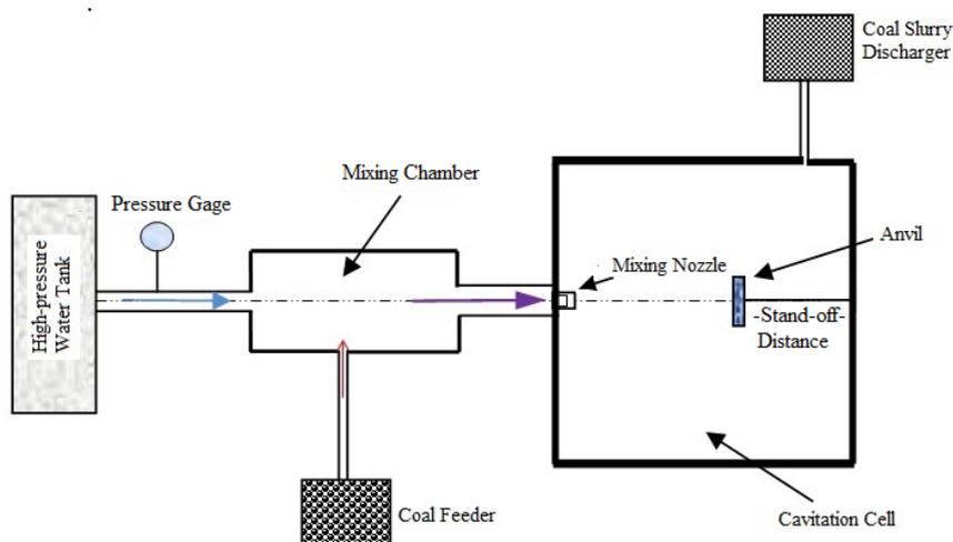
Fig. 1. Schematic of the high-pressure waterjet mill
