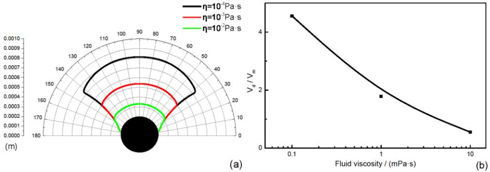
Fig. 5. Effect of the fluid viscosity on the saturated particle buildup: magnetic induction  $B_0 = 0.5$  T, matrix radius  $a = 0.2$  mm, particle radius  $b = 10$   $\mu\text{m}$
