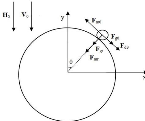
Fig. 1. Components of forces acting on spherical particle
