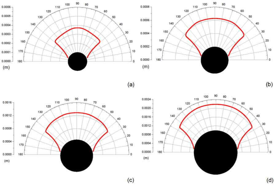
Fig. 8. Saturated buildup of particles of radius 15 μm on the matrices with radii of (a) 0.1 mm, (b) 0.2 mm; (c) 0.5 mm and (d) 1.0 mm
