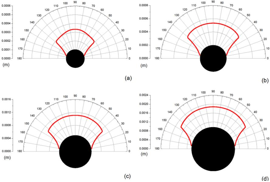
Fig. 9. Saturated buildup of particles of radius 10 μm on the matrices with radii of (a) 0.1 mm, (b) 0.2 mm; (c) 0.5 mm and (d) 1.0 mm
