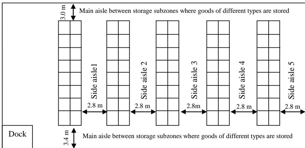
Fig. 5. The plan of warehousing zone for the beverages
