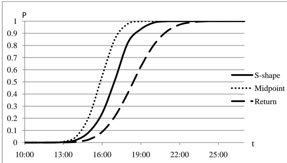
Fig. 6. Cumulative distribution function of order picking times (only forklifts work time)
