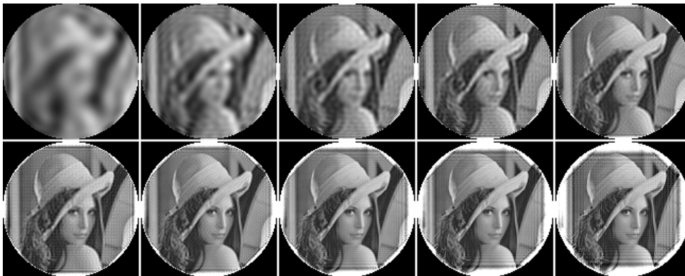
Figure 5.8: Image reconstruction from ZMs computed in the Cartesian coordinate system. First row from left to right: images reconstructed from ZMs up to order 20, 40, 60, 80 and 100 respectively. Second row from left to right: images reconstructed from ZMs up to order 120, 140, 160, 180 and 200, respectively
