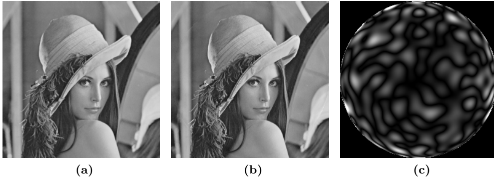
Figure 7.5: An example of using the proposed algorithm. (a) Original Lena image of size 256 \times 256 . (b) Lena watermarked with 128 bits. (c) Exaggerated difference of (b) and (a)
