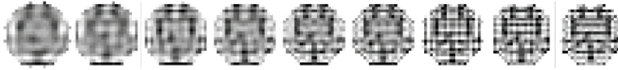
Figure 3.9: Reconstructed patterns of the character C_1 based on the Zernike moments of order 14, 16, 18, 20, 22, 24, 26, 28, and 30
