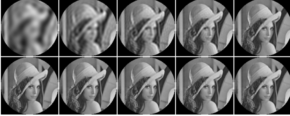
Figure 5.9: Image reconstruction from ZMs computed in the polar coordinate system. First row from left to right: images reconstructed from ZMs up to order 20, 40, 60, 80 and 100 respectively. Second row from left to right: images reconstructed from ZMs up to order 120, 140, 160, 180 and 200, respectively
