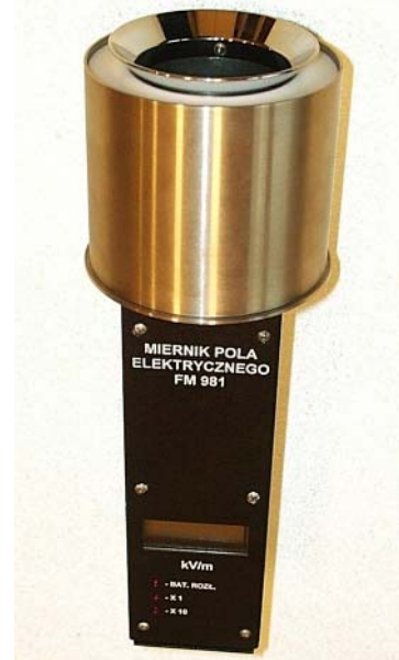
Fig. 4.4. Fieldmeter (FM981) – Faraday cage measuring set for total charge in loose materials General view
