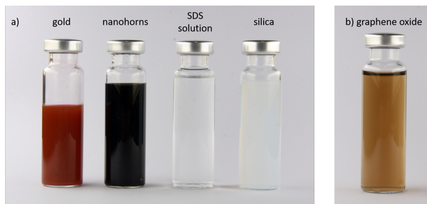
Figure 4.1: Investigated working fluids: a) gold nanofluid, nanohorn nanofluid, water solution of SDS, silica nanofluid, b) graphene oxide nanofluid
