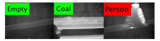
Fig. 12. Results of the person detection (Uth, Tokarczyk 2019)
