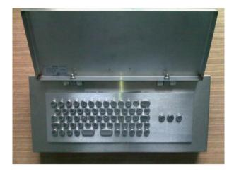
Fig. 3. Intrinsically safe keyboard type PCK001
