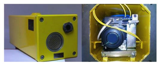
Figure 7. View of the thermal imaging camera system in explosion-proof version after removal of the front cover (left), thermal imaging camera in explosion-proof housing (right)
