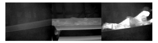
Fig. 10. Exemplary thermal images for categories empty belt conveyor (left), belt conveyor with coal (middle); person on belt conveyor (right) (Uth 2019)
