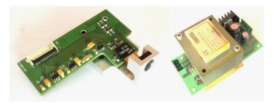
Figure 6. Video camera with electronic system (left), power supply for thermal imaging camera (right)
