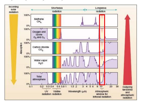
Fig. 1. Atmospheric absorption of incoming shortwave (left) and outgoing longwave (right) radiation (https://cimss.ssec.wisc.edu/sage/meteorology/lesson1/AtmAbsorbtion.htm, 2019)
