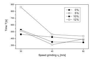
Fig. 6. Grinding material volume ( $Q_w = 1200 \text{ mm}^3$ ) removal time as a function of wheel speed grinding.
