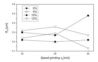
Fig. 7. Roughness of grinded workpieces surface, expressed by  $R_a$  parameter as a function of wheel speed grinding.
