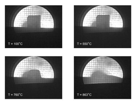
Fig. 2. Wetting of bubble alumina substrates by vitrified bond Pb21k.
