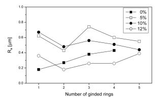
Fig. 9. Roughness of grinded work pieces surface, expressed by  $R_a$  parameter as a function of grinded rings number.
