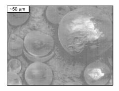
Fig. 3. Microphotographs of magnesium aluminosilicate microgranules, SEM, magn. 1000x.
