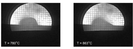
Fig. 4. Wetting of magnesium aluminosilicate substrate by Pb21K vitrified bond.
