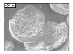
Fig. 1. Microphotographs of bubble alumina grains, SEM, magn. 1000x.
