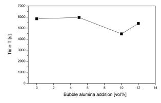
Fig. 8. Grinding material volume  $(Q_w - 18000 \text{ mm}^3)$  removal time as a function of bubble alumina percentage participation.
