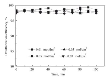
Fig. 12. Effect of Fe(II)EDTA concentration on SO<sub>2</sub> removal efficiency (25 °C, concentrations of: pH 5–6, NO<sub>x</sub> – 400 mg·m<sup>-3</sup>, SO<sub>2</sub> – 1400 mg·m<sup>-3</sup>, O<sub>2</sub> – 20%, 2.0 V, 15 A)
