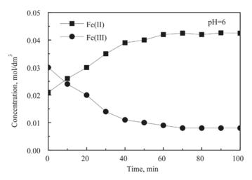
Fig. 9. Fe(II) and Fe(III) concentrations in ammonia-Fe(II)EDTA solution during electrochemical regeneration (25 °C, pH 6, concentrations of: Fe(II)EDTA – 0.05 mol·dm<sup>-3</sup>, NO<sub>x</sub> – 400 mg·m<sup>-3</sup>, SO<sub>2</sub> – 1400 mg·m<sup>-3</sup>, O<sub>2</sub> – 20%, 2.0 V, 15 A)
