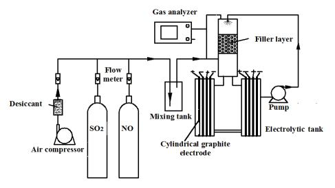
and the flow rate of air was controlled by a rotameter. The simulated flue gas was mixed in a tank to improve the distribution uniformity before entering the spray reactor.
