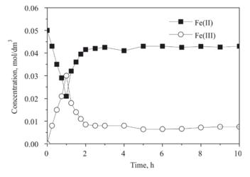
Fig. 17. Fe(II) and Fe(III) concentrations in ammonia-Fe(II)EDTA solution during electrochemical regeneration process (25 °C, concentrations of: Fe(II)EDTA – 0.05 mol·dm<sup>-3</sup>, O<sub>2</sub> – 18%, 2.1 V, 62 A)
