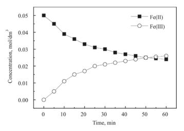
Fig. 7. Effect of reaction time on F(II) and Fe(III) concentrations in ammonia-Fe(II)EDTA (25 °C, pH 5–6, concentrations of:
