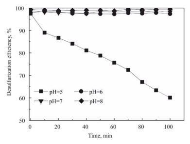
Fig. 10. Effect of pH on SO<sub>2</sub> removal efficiency (25 °C, concentrations of: Fe(II)EDTA – 0.05 mol·dm<sup>-3</sup>, NO<sub>x</sub> – 400 mg·m<sup>-3</sup>, SO<sub>2</sub> – 1400 mg·m<sup>-3</sup>, O<sub>2</sub> – 20%, 2.0 V, 15 A)
