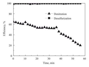
Fig. 6. Simultaneous removal of SO<sub>2</sub> and NO<sub>x</sub> with ammonia-Fe(II)EDTA (25 °C, pH 5–6, concentrations of: Fe(II)EDTA – 0.05 mol·dm<sup>-3</sup>, NO<sub>x</sub> – 400 mg·m<sup>-3</sup>, SO<sub>2</sub> – 1400 mg·m<sup>-3</sup>, O<sub>2</sub> – 20%)
