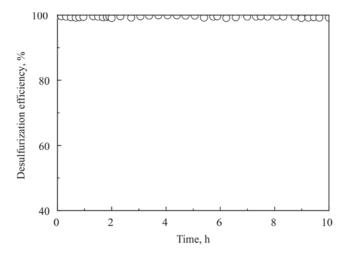
Fig. 18. Desulfurization efficiency in a pilot-scale reactor (25 °C, concentrations of: Fe(II)EDTA – 0.05 mol $\cdot$ dm<sup>-3</sup>, pH 5–6, O<sub>2</sub> – 18%, 2.1 V, 62 A)
