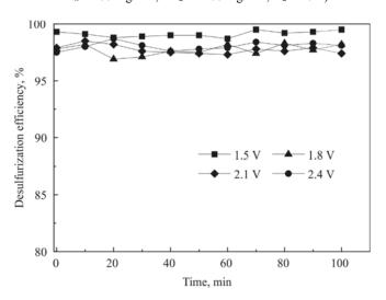
Fig. 15. Effect of voltage on SO<sub>2</sub> removal efficiency (25 °C, concentrations of: Fe(II)EDTA – 0.05 mol·dm<sup>-3</sup>, pH 5–6, NO<sub>x</sub> – 400 mg·m<sup>-3</sup>, SO<sub>2</sub> – 1400 mg·m<sup>-3</sup>, O<sub>2</sub> – 20%)
