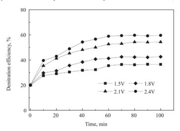
Fig. 13. Effect of voltage on NO<sub>x</sub> removal efficiency (25 °C, concentrations of: Fe(II)EDTA – 0.05 mol·dm<sup>-3</sup>, pH 5–6, NO<sub>x</sub> – 400 mg·m<sup>-3</sup>, SO<sub>2</sub> – 1400 mg·m<sup>-3</sup>, O<sub>2</sub> – 20%)
