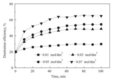
Fig. 11. Effect of Fe(II)EDTA concentration on NO<sub>x</sub> removal efficiency (25 °C, concentrations of: pH 5–6, NO<sub>x</sub> – 400 mg·m<sup>-3</sup>, SO<sub>2</sub> – 1400 mg·m<sup>-3</sup>, O<sub>2</sub> – 20%, 2.0 V, 15 A)
