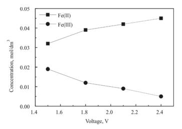
Fig. 14. Effect of voltage on Fe(II) and Fe(III) concentrations in ammonia-Fe(II)EDTA solution (25 °C, concentrations of: Fe(II)EDTA – 0.05 mol·dm<sup>-3</sup>, pH 5–6, NO<sub>x</sub> – 400 mg·m<sup>-3</sup>, SO<sub>2</sub> – 1400 mg·m<sup>-3</sup>, O<sub>2</sub> – 20%)
