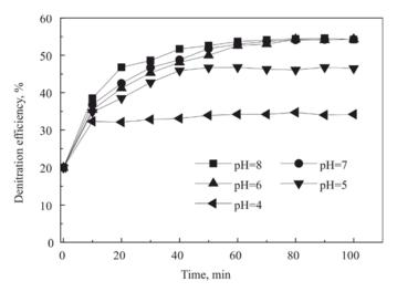
Fig. 8. Effect of pH on NO<sub>x</sub> removal efficiency (25 °C, concentrations of: Fe(II)EDTA – 0.05 mol·dm<sup>-3</sup>, NO<sub>x</sub> – 400 mg·m<sup>-3</sup>, SO<sub>2</sub> – 1400 mg·m<sup>-3</sup>, O<sub>2</sub> – 20%, 2.0 V, 15 A)
