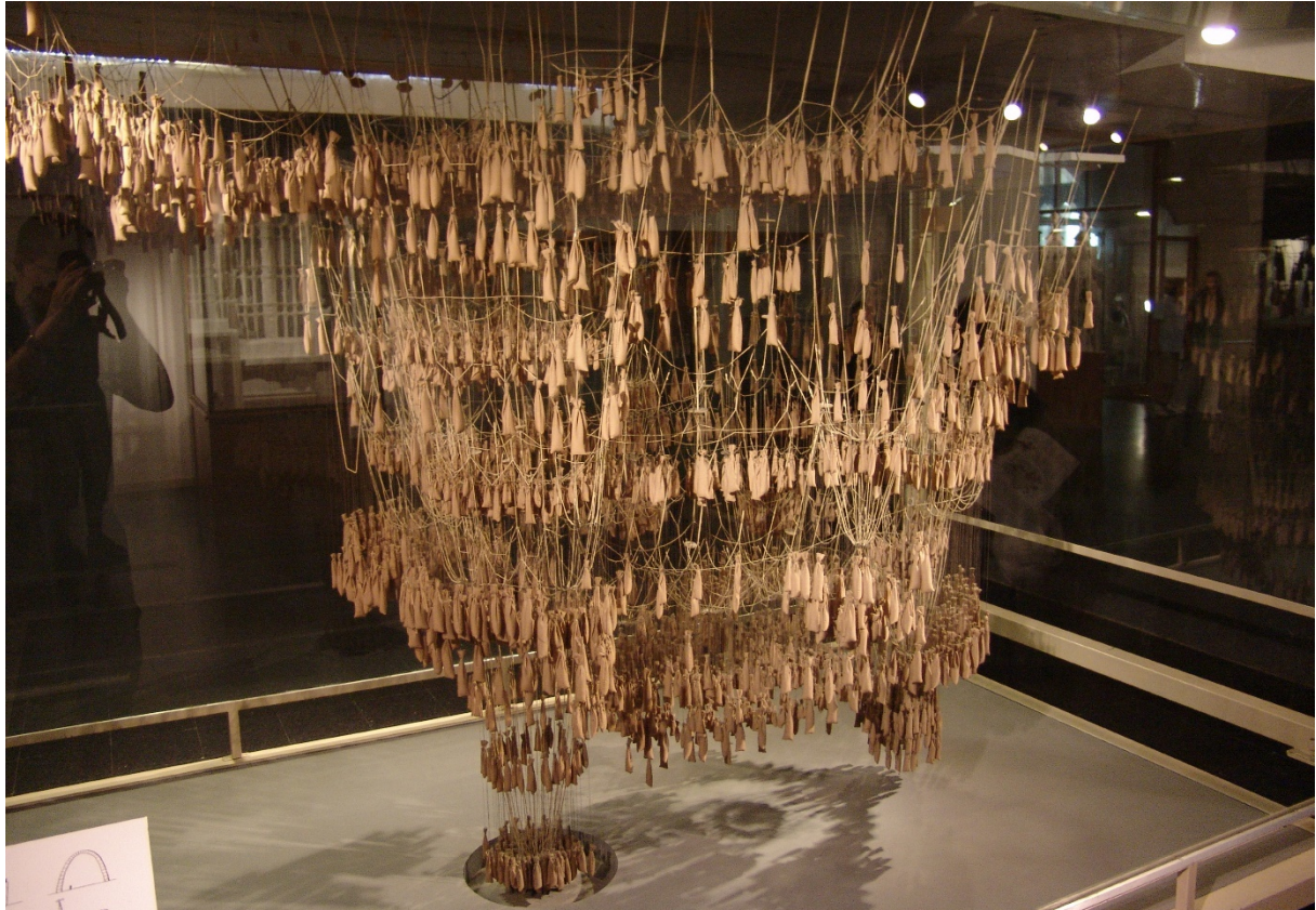
Fig. 2.5 Catenary model of the structural system of the Sagrada Familia. 14
