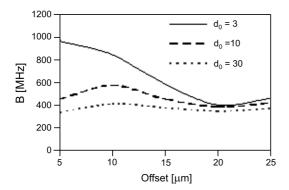
Fig. 2. Modal bandwidth in the presence of modal filtering with the filter (16) and for a distorted profile (15), launch beam diameter is 9  $\mu$ m,  $d(x) = d_0 = \text{const} [1/\text{km}]$ .
