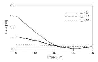
Fig. 4. Modal filtering loss for the data from Fig. 3 for various coupling coefficients  $d(x) = d_0 [1/\text{km}]$ .
