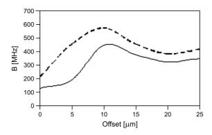
Fig. 3. Modal bandwidth in the absence of modal filtering (solid line), and in its presence (dashed line). Modal filtering is with the filter (16) and for the distorted profile (15), launch beam diameter is 9  $\mu$ m,  $d(x) = d_0 = 10$  [1/km]. Modal filtering loss does not exceed here 6.1 dB.
