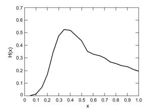
Fig. 5. Transfer function H(x) realized in a MM fiber ( $\lambda = 0.78 \,\mu\text{m}$ ,  $D = 50 \,\mu\text{m}$ , g = 2, NA = 0.2,  $n_1 = 1.48$ ) by a circular diaphragm located at the fiber end that is opaque for  $r < 10 \,\mu\text{m}$  and for  $r > 15 \,\mu\text{m}$ , and transparent elsewhere.
