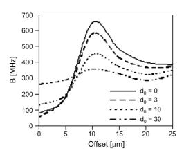
Fig. 1. Modal bandwidth *B*, versus offset: the exciting beam diameter is 9  $\mu$ m,  $d(x) = d_0 = \text{const} [1/\text{km}]$ . The profile is distorted according to (15): h = 0.5 and  $x_0 = 0.05$ .
