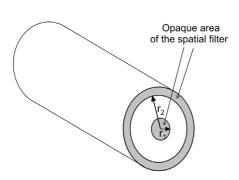
Fig. 6. View of the fiber core end surface. A spatial filter that realizes the transfer function in Fig. 5 is applied. The fiber cladding is not shown.
