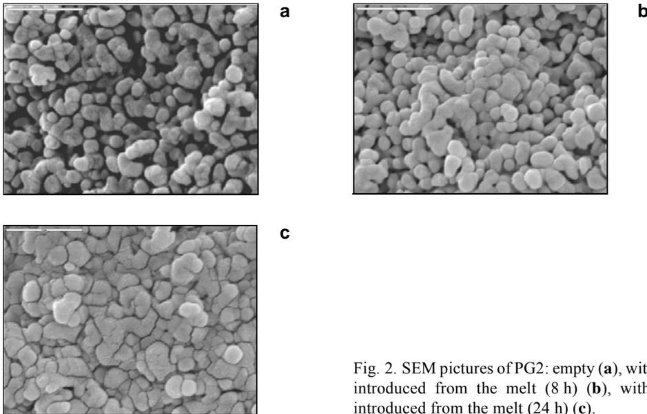
Fig. 2. SEM pictures of PG2: empty (a), with  $\text{NaNO}_2$  introduced from the melt (8 h) (b), with  $\text{NaNO}_2$  introduced from the melt (24 h) (c).
