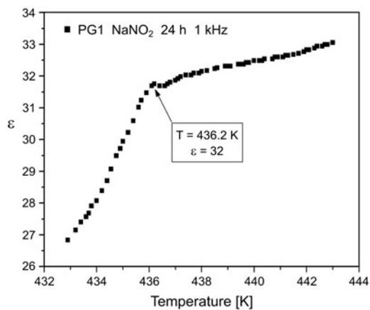
Fig. 8. Temperature dependence of dielectric permittivity of PG1 with  $\text{NaNO}_2$  introduced from the melt (filling time 24 h). The measurements have been carried out in 20 days after the sample preparation.
