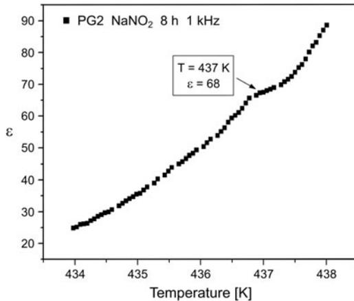
Fig. 6. Temperature dependence of dielectric permittivity of PG2 with  $\text{NaNO}_2$  introduced from the melt (filling time 8 h) at frequency 1 kHz.
