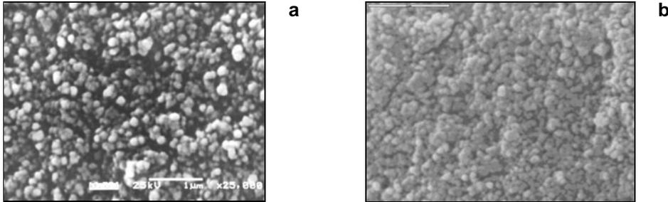
Fig. 1. SEM pictures of PG1: empty (a), with  $\text{NaNO}_2$  introduced from the melt (24 h) (b).
