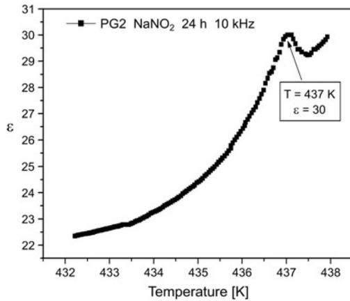
Fig. 7. Temperature dependence of dielectric permittivity of PG2 with  $\text{NaNO}_2$  introduced from the melt (filling time 24 h, fast cooling) at frequency 10 kHz.
