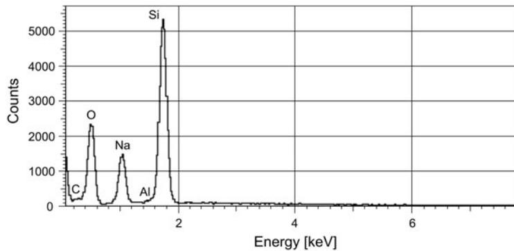
Fig. 3. EDS spectrum of PG2 with  $\text{NaNO}_2$  introduced from the melt (filling time 24 h).
