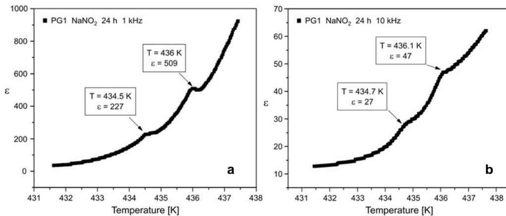
Fig. 4. Temperature dependences of dielectric permittivity of PG1 with  $\text{NaNO}_2$  introduced from the melt (filling time 24 h) at frequencies 1 kHz (a) and 10 kHz (b).
