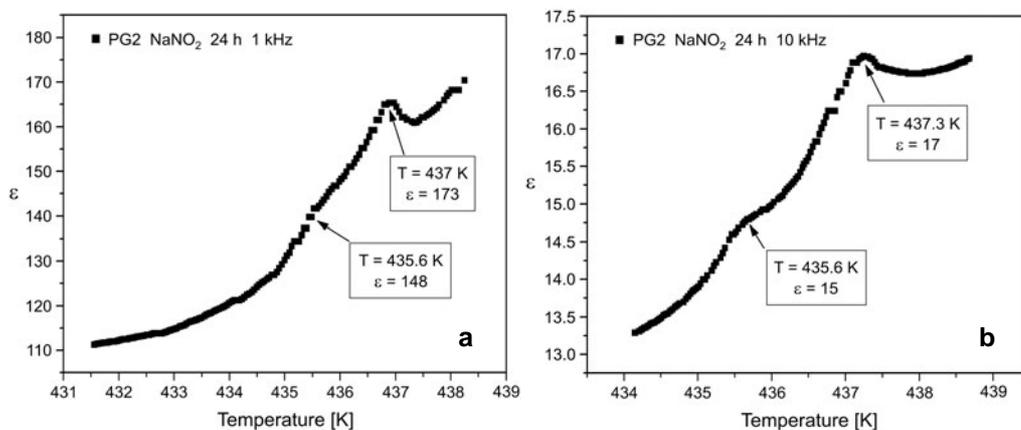
Fig. 5. Temperature dependences of dielectric permittivity of PG2 with  $\text{NaNO}_2$  introduced from the melt (filling time 24 h) at frequencies 1 kHz (a) and 10 kHz (b).
