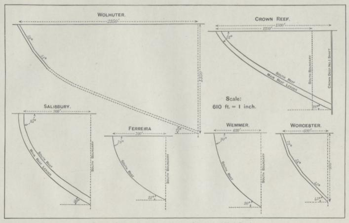
FIG. 47.—Diagrams illustrating the Decrease of the Angle of Dip in Depth.
