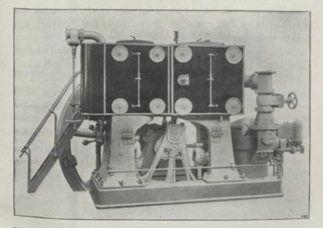
MILL ENGINE in use at the Henry Nourse. Compound-condensing—King type. Corliss valve gear. Steam cylinders, 19 in. and 30 in., diameter ; stroke, 42 in.; revolutions per minute, 75; indicated horse-power, 330. Automatic cut-off in high-pressure cylinder to 70 per cent of the stroke. Hand cut-off in the low-pressure cylinder. Both cylinders steam-jacketed.
