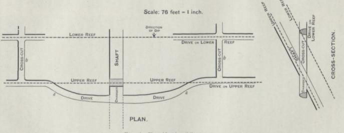
FIG. 56.-Plan of Levels and Cross-cuts.
