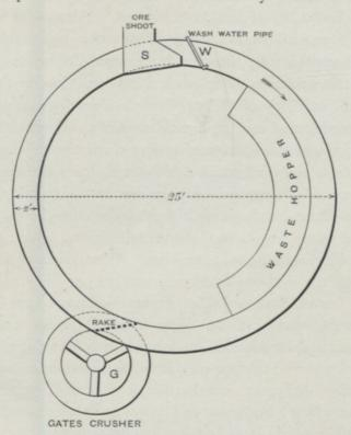
FIG. 67.-Plan of Circular Sorting-Table at the City and Suburban Company's Mine.
