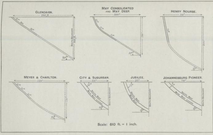
FIG. 48.—Diagrams illustrating the Decrease of the Angle of Dip in Depth—Continued.
