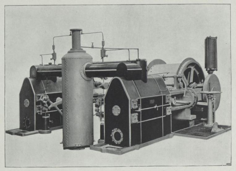
PLATE XII. - WINDING ENGINE, 20" × 48", IN USE AT THE JUMPERS DEEP.
