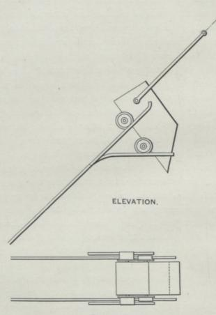
PLAN. FIG. 62—Plan and Section of a Self-dumping Skip.
