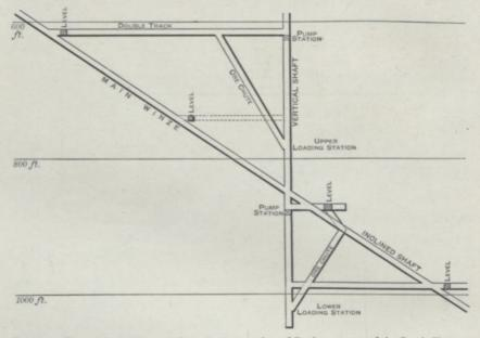
FIG. 60.—Proposed Arrangement for reducing number of Stations at one of the South Simmer and Jack Shafts.
