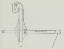
FIG. 68.-Jockey used in Endless Rope-haulage.
