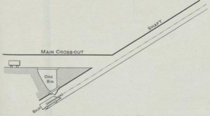
FIG. 58.—Arrangement for loading Skips.
