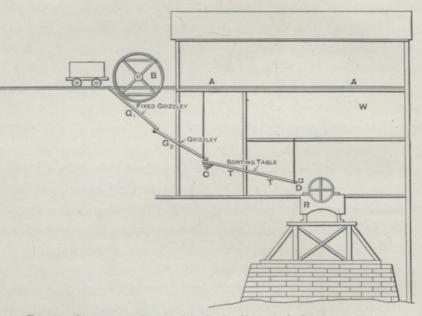
FIG. 66.—Diagrammatic Section of the Sorting-House at the Roodepoort United Main Reef Company's Mine.
