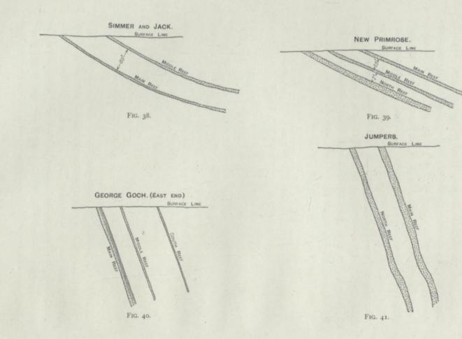
lie the payable ore-bodies, which are taken out in one big stope. They consist of two main bodies. The uppermost of these (Middle Reef) is distinguished by a slaty parting on the foot-wall. It consists of some 15 to 20 inches of pay ore. In the western part of the mine it is split up into two small leaders separated by a seam of sandstone. Of these the foot-wall leader, although small, is very rich.
