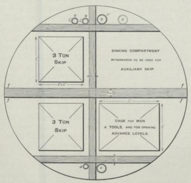
FIG. 53.-Section of Round Shaft at the Langlaagte Royal.
