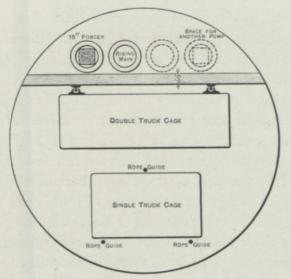
FIG. 52.-Section of Round Shaft at the New Primrose.
