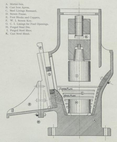
FIG. 76.—Section of the Mortar used at New Croesus Mine, showing Stamp Head, Shoe, Die, and other parts.
