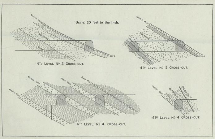
FIG. 5.-Sections of the Reefs worked in the New Primrose Mine.
