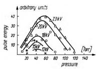
Fig. 3. The laser pulse energy as a function of gas pressure obtained without back mirror
