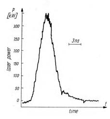
Fig. 5. Typical shape of the laser pulse obtained by using sampling method
