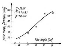
Fig. 4. The laser pulse energy as a function of tube length obtained for U = 23 kVand p = 50 Torr of nitrogen
