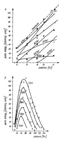
Fig. 2. The laser pulse energy a) as a function of applied voltage, b) as a function of gas pressure, obtained by using back mirror
