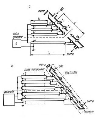
Fig. 1. Schematic diagram of the laser device with coaxial cables
