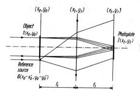
Fig. 1. Recording of Fourier-type hologram
