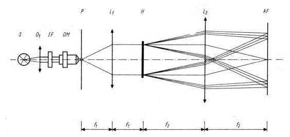
Fig. 3. Diagram of an experimental setup for partially coherent reconstruction of Fourier holograns
