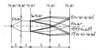
Fig. 2. Reconstruction of Fourier-type hologram
