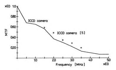
Fig. 9. MTF of ICCD camera calculated from edge response.
