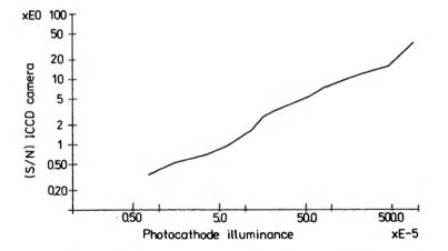
Fig. 8. S/N ratio for ICCD camera against photocathode illuminance
