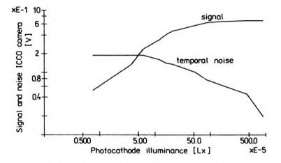
Fig. 7. Signal and noise of ICCD camera against photocathode illuminance
