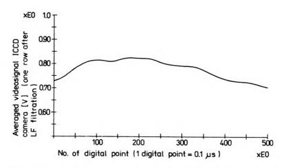
Fig. 12. Result of low frequency digital filtering of videosignal presented in Fig. 11
