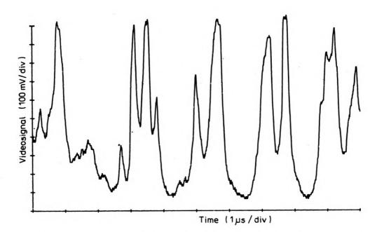
Fig. 3. Photon noise on digital oscilloscope display in the measurement of CICCD signal with 0.5 MHz test pattern
