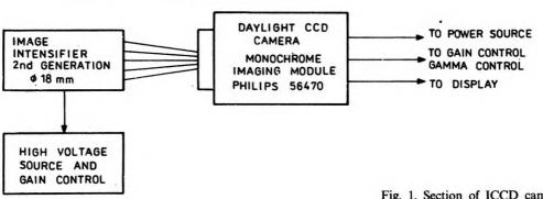
Fig. 1. Section of ICCD camera
