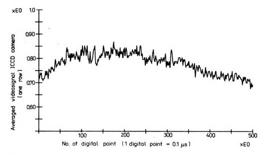
Fig. 11. Part of line of videosignal from ICCD camera. Temporal noise eliminated by applying AVERAGE mode
