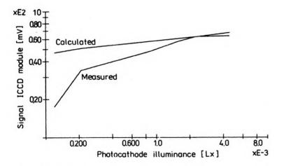
Fig. 5. Experimental measurement and theoretical prediction of ICCD modul signal against photocathode illuminance
