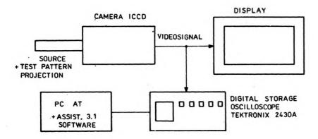
Fig. 2. Assembly for TV measurement
