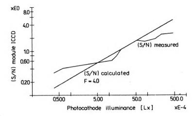
Fig. 6. Measurement of ICCD modul S/N ratio and calculation of S/N ratio against photocathode illuminance for F = 4.0
