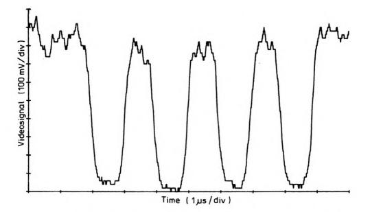
Fig. 4. Elimination of photon noise from videosignal with AVERAGING mode using TEKTRONIX 2430A digital oscilloscope
