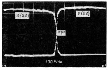
Fig. 1. Intensity changes of two competing lines as a function of laser frequency. "P" - equal-intensity point
