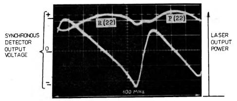
Fig. 3. Laser output power and simultaneous voltage from the synchronous detector as a function of laser frequency. The peak laser power is 2 W
