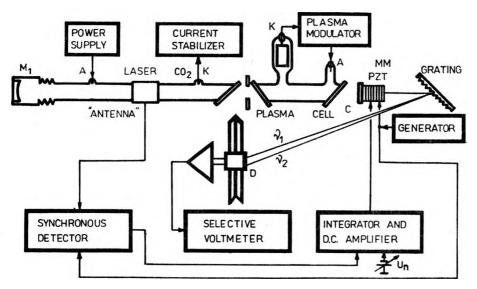
Fig. 2. Detailed schematic diagram of the plasma diagnostic setup
