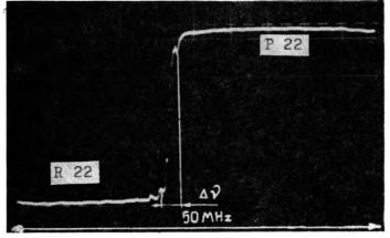
Fig. 4. Output voltage from differential detector as a function of laser frequency.  $\Delta v$  - competition interval
