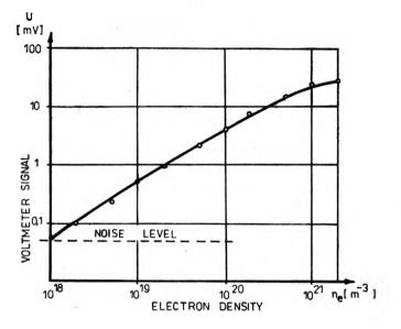
Fig. 5. Scaling curve of the plasma diagnostic setup
