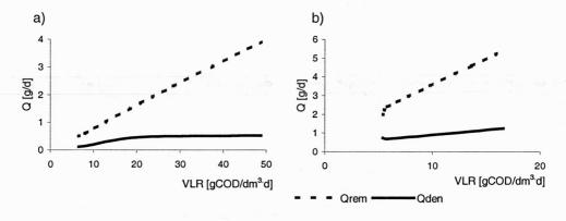
Fig. 2. Organic load removed by denitrification ( $Q_{den}$ ) versus VLR in reactors I (a) and II (b)
