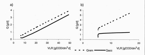
Fig. 4. Organic load accumulated intracellularly  $(Q_{acc})$  versus VLR in reactors I (a) and II (b)
