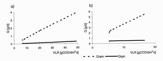
Fig. 3. Organic load used for biomass synthesis versus VLR in reactors I (a) and II (b)
