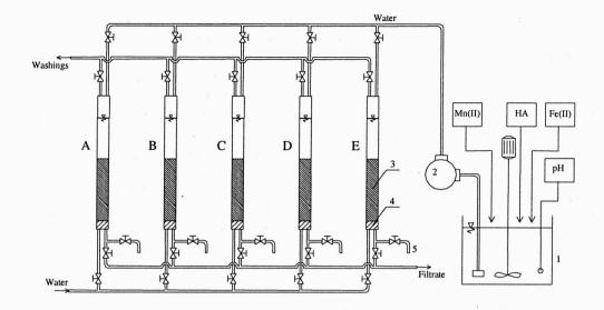
Fig. 1. Experimental set-up: 1 – raw water tank, 2 – dosing pump, 3 – filtration layer (active mass),
