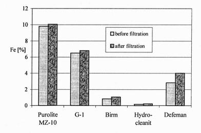
Fig. 5. Iron percent in active beds before and after filtration process
