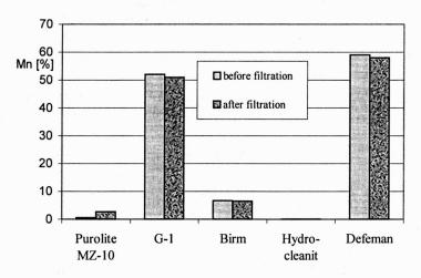
Fig. 4. Manganese percent in active beds before and after filtration process
