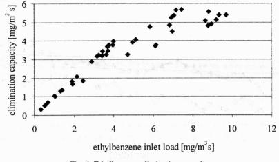
As it can be seen in figure 4, the maximum load of t thylbenzene was 7 mg/(m<sup>3</sup>·s). Further increase in the load does not increase the elimination capacity of the bed.
