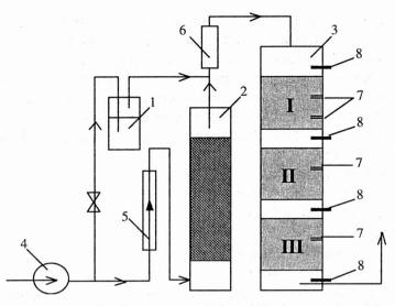
Fig. 1. The laboratory-scale biofiltration system used: *I* – bubbler for saturation of air with pollutant, *2* – air damping column, *3* – biofilter, *4* – pump, *5* – rotameter, *6* – mixing chamber, *7* – pipe connectors used for filter bed moisture control, *8* – pipe connectors for gas sampling
