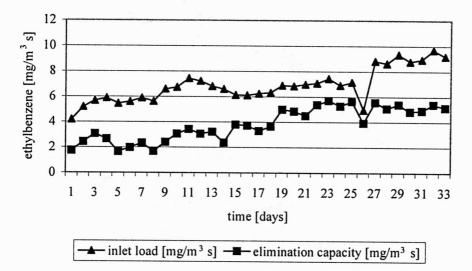
Fig. 2. Changes of the inlet concentration and of the ethylbenzene elimination capacity during the whole test series
