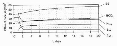
Fig. 11. Transition from the configuration A ( $V_{\text{NIT}} = 4500 \text{ m}^3$ , MLSS<sub>A</sub>  $\approx 3000 \text{ mg SS/dm}^3$ , SRT = 6 d) to the configuration B ( $V_{\text{NIT}} = 3000 \text{ m}^3$ ,  $V_{\text{DEN}} = 1500 \text{ m}^3$ , SRT = 9 d). Temperature = 15 °C, resultant MLSS<sub>B</sub>  $\approx 4100 \text{ mg SS/dm}^3$
