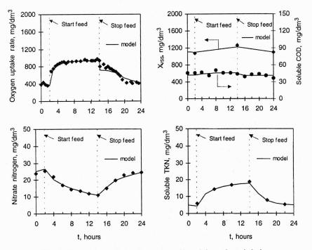
Fig. 3. Comparison of experimental results and the activated sludge model predictions under daily wave loading conditions [10]
