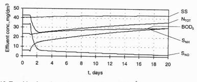
Fig. 10. Transition from the configuration A ( $V_{\text{NIT}} = 4500 \text{ m}^3$ , MLSS<sub>A</sub>  $\approx 3000 \text{ mg SS/dm}^3$ , SRT = 6 d) to the configuration B ( $V_{\text{NIT}} = 3000 \text{ m}^3$ ,  $V_{\text{DEN}} = 1500 \text{ m}^3$ , SRT = 6 d). Temperature = 15 °C, resultant MLSS<sub>B</sub>  $\approx 3200 \text{ mg SS/dm}^3$
