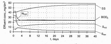
Fig. 14. Transition from the configuration A ( $V_{\text{NIT}} = 4500 \text{ m}^3$ , MLSS<sub>A</sub>  $\approx 3000 \text{ mg SS/dm}^3$ , SRT = 6 d) to the configuration C ( $V_{\text{NIT}} = 4000 \text{ m}^3$ ,  $V_{\text{DEN}} = 1500 \text{ m}^3$ , SRT = 12 d). Temperature = 15 °C, resultant MLSS<sub>C</sub>  $\approx 4300 \text{ mg SS/dm}^3$
