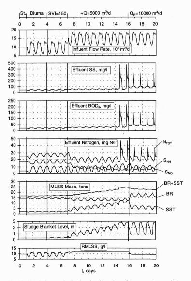
Fig. 19. Simulation results for the plant E under various operating conditions
