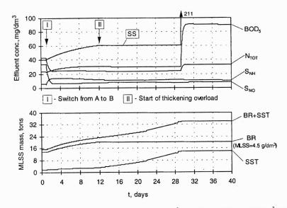
Fig. 12. Transition from the configuration A ( $V_{\text{NIT}} = 4500 \text{ m}^3$ , MLSS<sub>A</sub>  $\approx 3000 \text{ mg SS/dm}^3$ , SRT = 6 d) to the configuration B ( $V_{\text{NIT}} = 3000 \text{ m}^3$ ,  $V_{\text{DEN}} = 1500 \text{ m}^3$ , target SRT = 12 d). Temperature = 15 °C
