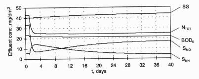
Fig. 18. Transition from the configuration A ( $V_{\text{NIT}} = 4500 \text{ m}^3$ , MLSS<sub>A</sub>  $\approx 3000 \text{ mg SS/dm}^3$ ,  $V_{\text{SST}} = 1500 \text{ m}^3$ , SRT = 6 d) to the configuration E ( $V_{\text{NIT}} = 3000 \text{ m}^3$ ,  $V_{\text{DEN}} = 1500 \text{ m}^3$ ,  $V_{\text{SST}} = 1500 \text{ m}^3$ ,  $V_{\text{PST}} = 1000 \text{ m}^3$ , SRT = 12 d). Temperature = 15 °C, resultant MLSS<sub>E</sub>  $\approx 3200 \text{ mg SS/dm}^3$
