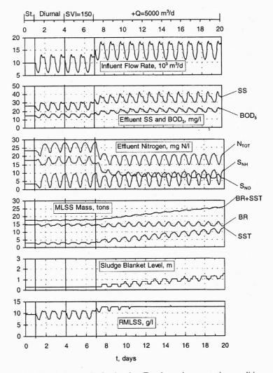
Fig. 21. Simulation results for the plant F under various operating conditions
