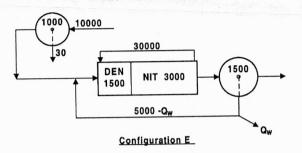
Fig. 16. Configuration E of the upgraded plant
