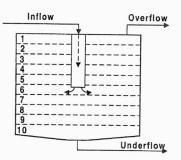
Fig. 4. Layered final settler model
