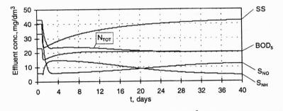
Fig. 17. Transition from the configuration A ( $V_{\text{NIT}} = 4500 \text{ m}^3$ , MLSS<sub>A</sub>  $\approx 3000 \text{ mg SS/dm}^3$ ,  $V_{\text{SST}} = 1500 \text{ m}^3$ , SRT = 6 d) to the configuration D ( $V_{\text{NIT}} = 3000 \text{ m}^3$ ,  $V_{\text{DEN}} = 1500 \text{ m}^3$ ,  $V_{\text{SST}} = 2500 \text{ m}^3$ , SRT = 12 d). Temperature = 15 °C, resultant MLSS<sub>D</sub>  $\approx 5000 \text{ mg SS/dm}^3$
