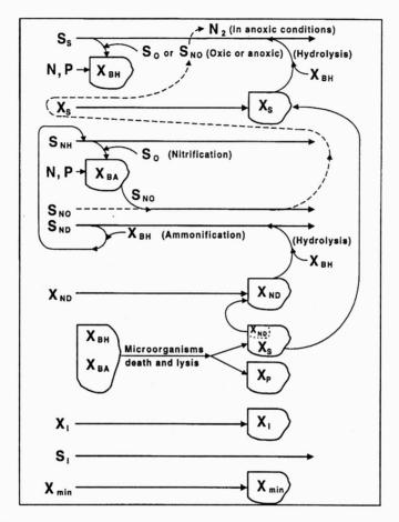
Fig. 2. Scheme of sewage pollutant transformation in activated sludge process
