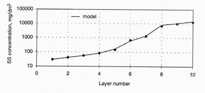
Fig. 5. Comparison of the observed and simulated SS concentration profiles in a full-scale secondary settling tank [11]
