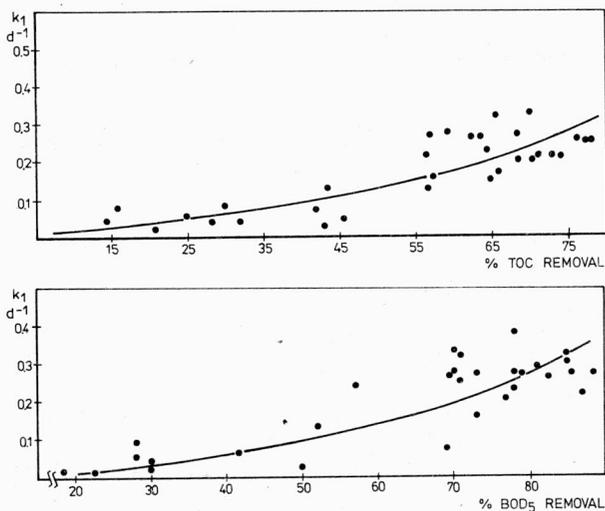
Fig. 5. Reaction rate coefficient constant  $k_1$  versus the degrees of TOC and  $BOD_5$  removals
