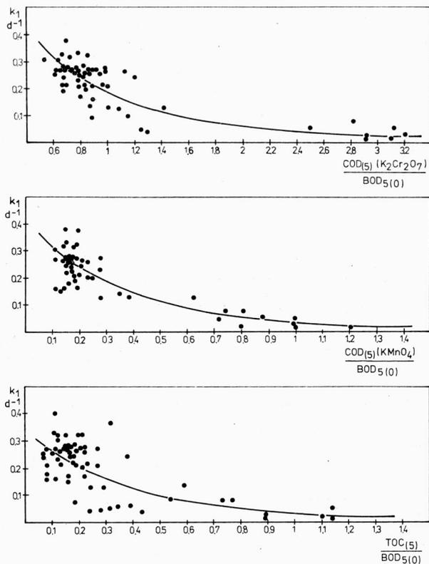
Fig. 6. Reaction rate coefficient constant  $k_1$  versus the ratios of COD and TOC (after five days of aeration) to  $BOD_5$  (non-treated samples)
