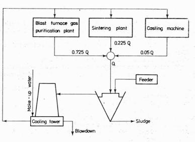
Fig. 2. The diagram of joining the cycles of blast furnace gas purification plant, sintering plant and the casting machines into integrated system
