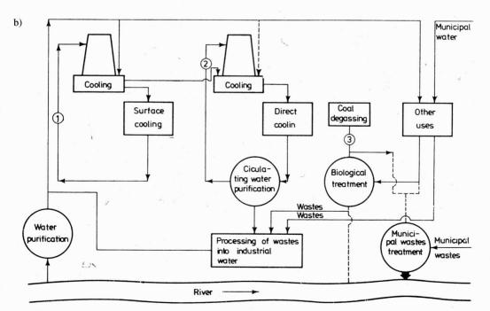
Fig. 1. Layout of water and wastewater management in partially closed cycle (1a) and in the fully closed (1b)
