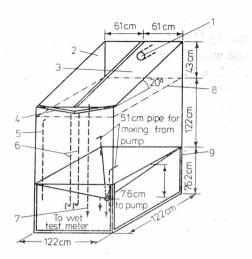
Fig. 2. Schematic of solar-heated methane generator
