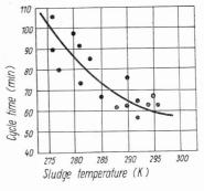
Fig. 13. Effect of temperature on pressure filter cycle time Antwerp waterworks sludge
