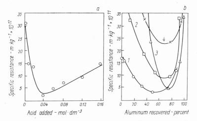
Fig. 17. Effects of acidification and subsequent coagulant recovery on the filterability of waterworks chemical sludges:
