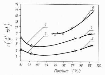
Fig. 6. Influence of initial water contents in waterworks sludges on their specific resistance r:
