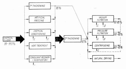
Fig. 1. Alternative methods of dewatering chemical sludges. (In brackets: sludge moisture usually attained); c – indicates possibility of coagulant addition; p – precoat may be applied
