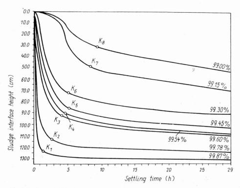
Fig. 2. Settling and thickening curves for alum sludge from water treatment plant at Tomaszów, for various initial solids content. Points K denote the beginning of thickening phase
