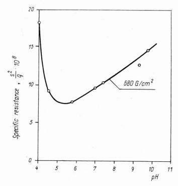
Fig. 7. Effect of varying pH on filtrability of Tomaszów waterworks alum sludge at initial moisture of 98.2%
