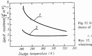
Fig. 12. Influence of temperature on specific resislance of Wrocław waterworks sludge at initial solids 95.02%,
