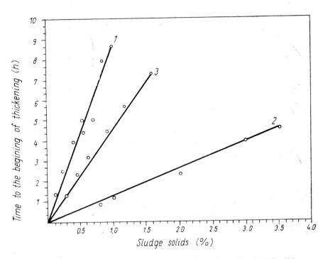
Fig. 3. Time to the beginning of thickening of sludges with various initial solids concentrations:
