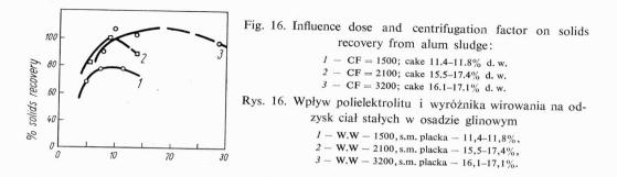
for contribugation efficiency. At the present high level of technology of vacuum filtration the centrifuge will become competitive only after the improvement of centrate quality (solids recovery) and low cake solids attained usually with sludges from chemical coagulation.
