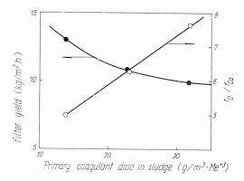
Fig. 9. Filtration of primary wastewater coagulation sludge, conditioned with lime, at various primary coagulant doses
