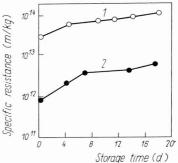
Fig. 8. Change of specific resistance as the result of aging; *I* - raw wastewater coagulation sludge, *2* - the same sludge after 30 days of aerobic stabilization
