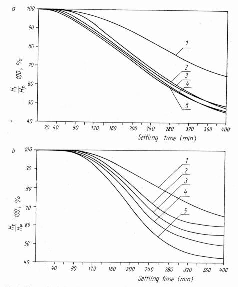
Fig. 4. Effects of polyelectrolytes on settling and thickening of sludge from Tomaszów waterworks at initial water contents of 99.11%:
