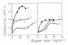
An optimum polyelectrolyte dose for the post-coagulation sludge increases with the increase of the solids contents of the sludge applied to the filter and with the increase of filter yield. Similar relationships are found for wastewater chemical sludges, which should always be conditioned with polymers since they contain very difficult to dewater solids built of phosphorous compounds.
