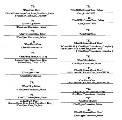
Fig. 4. State transitions for source client.
