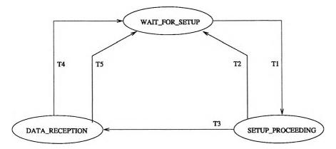
Fig. 5. State diagram for destination client.
