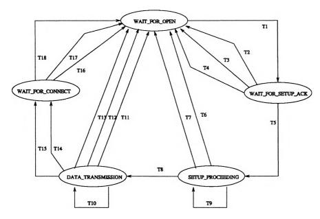
Fig. 3. State diagram for source client.
