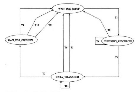
Fig. 7. State diagram for ingress switch.
