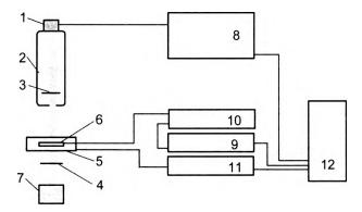
Fig. 1. Block scheme of the electro-optic measuring set-up: 1 - silicone diode photodetector, 2 - polarizing microscope, 3 - analyzer, 4 - polarizer, 5 - hot stage, 6 - PDLC sample, 7 - halogen lamp, 8 - oscilloscope, 9 - signal generator, 10 - voltage amplifier, 11 - hot-stage driver, 12 - driving PC.
