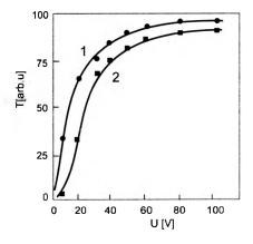
Fig. 9. Static electro-optical characteristics of PDLC containing: 1 - W-104 and 2 - W-101 mixtures; T = 40 °C; film thickness 8 µm, mean droplet volume  $\sim 15 \text{ µm}^3$ , mean aspect ratio  $\sim 10$ .
