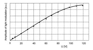
Fig. 3. Amplitude of light modulation vs. applied voltage for PDLC containing SmC $^{\bullet}_{\Lambda}$  phase of W-104 at 30 °C, mean droplet volume ~15  $\mu$ m<sup>3</sup>, mean droplet aspect ratio ~8.
