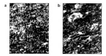
Fig. 4. Microscopic view of the PDLC film containing SmC<sub>A</sub> phase of W-104 at 75 °C. a – off-state, b – on state; film thickness 8  $\mu$ m, mean droplet volume ~15  $\mu$ m<sup>3</sup> mean droplet aspect ratio 8.
