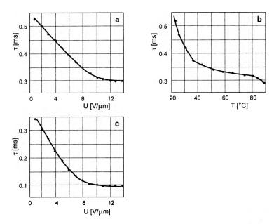
Fig. 8. Dependence of total switching time PDLC containing:  $SmC_A^{\bullet}$  phase of W-104 mixture on: a – applied voltage (at T=30 °C), b – temperature (at U=4 V), c –  $SmC^{\bullet}$  of the same mixture on applied voltage, T=85.5 °C; film thickness 8  $\mu$ m, mean droplet volume  $\sim 15 \,\mu$ m<sup>3</sup>, mean apect ratio  $\sim 10$ .
