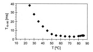
Fig. 7. Response time of PDLC film containing 20% b.w. of W-101A mixture vs. temperature; film thickness 8  $\mu$ m, mean droplet volume  $\sim 15 \mu$ m<sup>3</sup>, mean droplet aspect ratio 10.
