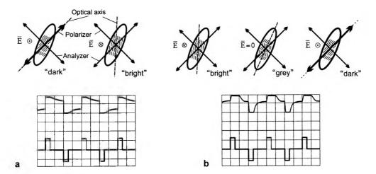
Fig. 2. Schematic oscilloscope view of saturated electro-optical switching of PDLC containing W-104 mixture by 100 Hz signal. Bistable switching of SmC $^{\bullet}$  phase at 85.5 °C (a), tristable switching of SmC $^{\bullet}$  phase at 75 °C (b), mean droplet volume ~15  $\mu$ m<sup>3</sup>, mean droplet aspect ratio ~10.
