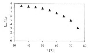
Fig. 5. Optical contrast vs. temperature for PDLC film containing 20% by weight of W-101A mixture; film thickness 8  $\mu$ m, mean droplet volume ~15  $\mu$ m<sup>3</sup>, mean droplet aspect ratio 10.
