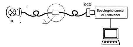
Fig. 1. Experimental set-up. IIL – halogen light source, L – coupling lens, F – optical fiber, S – container with urea solution and an optode, CCD – detector connected with the computer.
