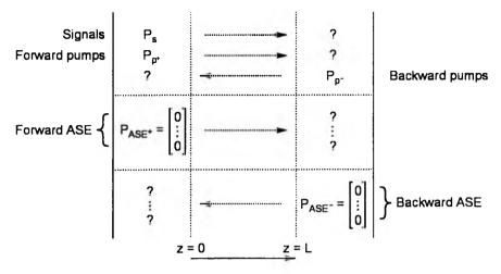
Fig. 1. Boundary conditions in EDFA. Dashed line arrows indicate propagation directions of light beams.
