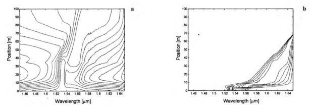
Fig. 5. Propagation of ASE noise in the forward (a) and backward (b) direction. The ASE noise power at a given position in the fibre was normalised to the maximum power of an ASE wavelength at this point. The z-axis is logarithmic. The EDF is 100 m long, the signal wavelength and pump wavelength is 1.60 mm and 0.98 mm, respectively. The signal power is 1 mW and the pump power is 100 mW.
