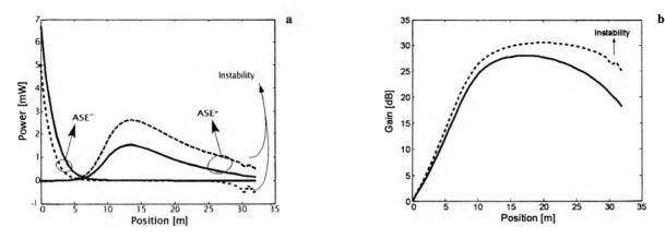
Fig. 4. Influence of the stabilization procedure on solution. The bold lines indicate solution after stabilization. Forward and backward ASE as a function of position in the fibre (a) and the gain as a function in the fibre (b).
