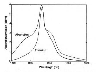
Fig. 2. Absorption and emission of a typical fibre given in Tab. 1.
