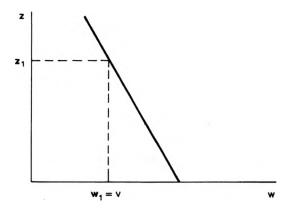
Fig. 10. Schematic presentation of the conditions for creation of an elevated aerosol layer (z - height, w - velocity of atmospheric upward motions, <math>v - fall velocity of aerosol,  $z_1 - height$  of aerosol layer ).
