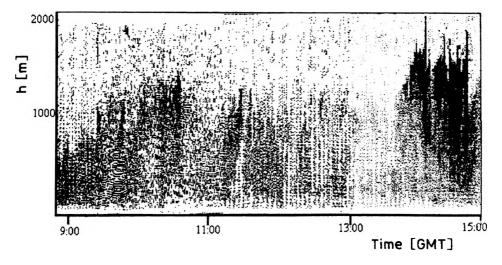
Fig. 1. Example of lidar record KEMA. Vertical axis - height, horizontal axis - time, backscatter intensity marked by grey-tone (June 16, 1995).
