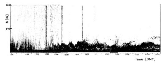
Fig. 3. Example of sodar record from March 10, 1995, 12:30 h to March 11, 1995, 03:20 h. Vertical axis – height, horizontal axis – time GMT. Note: 12:30-14:30 – convective plumes, 16:30-03:20 – ground-based inversion layer.
