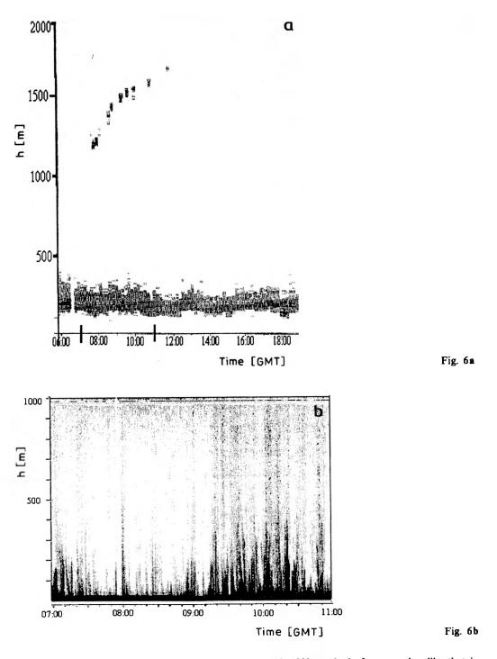
Fig. 6. Lidar-record (a) and sodar-record (b) of August 18, 1993; method of presentation like that in Figs. 2 and 3. At sodar record visible convective plumes.
