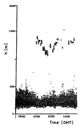
Fig. 2. Example of lidar record LIVERS, for description, see Fig. 1. Note: dead zone of observation (the lowest 100 m), ground-based aerosol layer, elevated aerosol layer (August 19, 1993).
