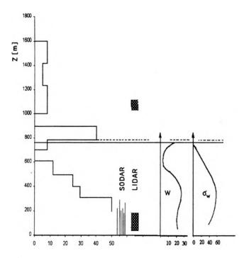
Fig. 5. Graphical representation of measurement results of August 18, 1993. Main graph (left) vertical axis – height, horizontal axis – SO<sub>2</sub> concentration  $[\mu g/m^3]$ , (mean layer concentrations). SODAR – height of sodar-observed convective plumes, LIDAR – lidar-observed aerosol layer, w – vertical velocity [cm/s] and its standard deviation  $\sigma_w$ .
