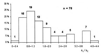
Fig. 4. Distribution of relation  $z_{\rm L}/z_{\rm C}$  (depth of the lidar-observed dust layer to the maximal height of sodar-observed convective structures). Measurements taken in Cracow, 1994-1996.
