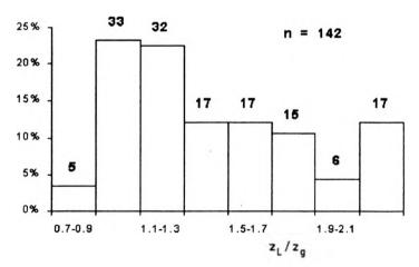
Fig. 7. Distribution of relation  $z_L/z_s$  (depth of lidar-observed dust layer divided by the depth of sodar-observed ground based echo layer). Measurements taken in Cracow, 1994–1996.
