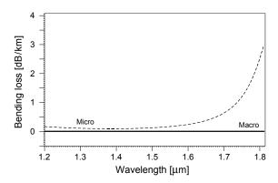
Fig. 5. Variations of bending loss vs. wavelength due to the addition of region  $R_2$  in refractive index profile.
