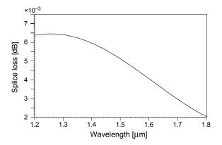
Fig. 12. Variations of splice loss via wavelength of our optimized fiber.
