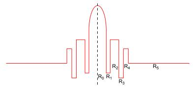
Fig. 1. Refractive index profile of the proposed optimized NZDSF.
