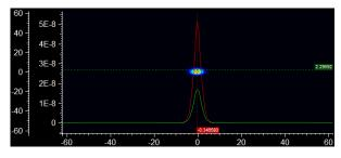
Fig. 27. Plot of the LP(0, 1) mode field vs. transverse dimensions of the fiber A.
