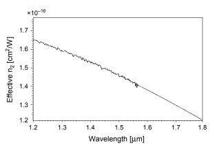
Fig. 10. Variations of  $n_2$  vs. wavelength of our optimized fiber.
