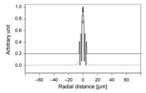
Fig. 26. Confinement in our optimized fiber B.
