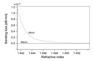
Fig. 24. Bending loss contribution vs. region  $R_4$  refractive index.
