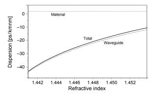
Fig. 23. Dispersion contribution vs. region  $R_4$  refractive index.
