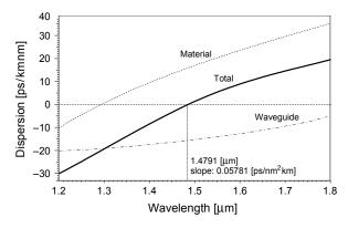
Fig. 8. Variations of dispersion vs. wavelength of our optimized fiber.
