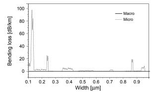
Fig. 22. Bending loss contribution vs. region  $R_4$  width.
