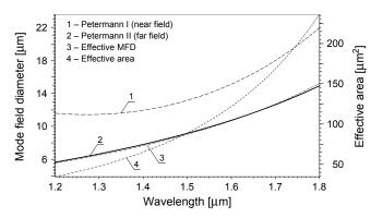
Fig. 9. Variations of effective area and MFD vs. wavelength of our optimized fiber.
