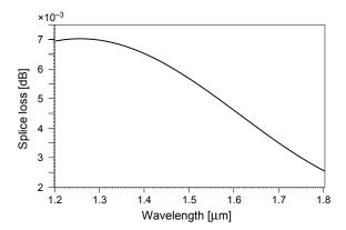
Fig. 6. Variations of splice loss vs. wavelength due to the addition of region  $R_2$  in refractive index profile.
