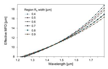
Fig. 20. Effective MFD vs. wavelength.
