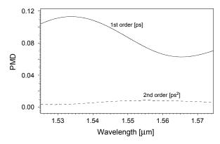
Fig. 4. Variations of PMD vs. wavelength due to the addition of region  $R_2$  refractive index profile.
