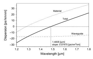
Fig. 3. Variations of dispersion vs. wavelength due to the addition of region  $R_2$  in refractive index profile.
